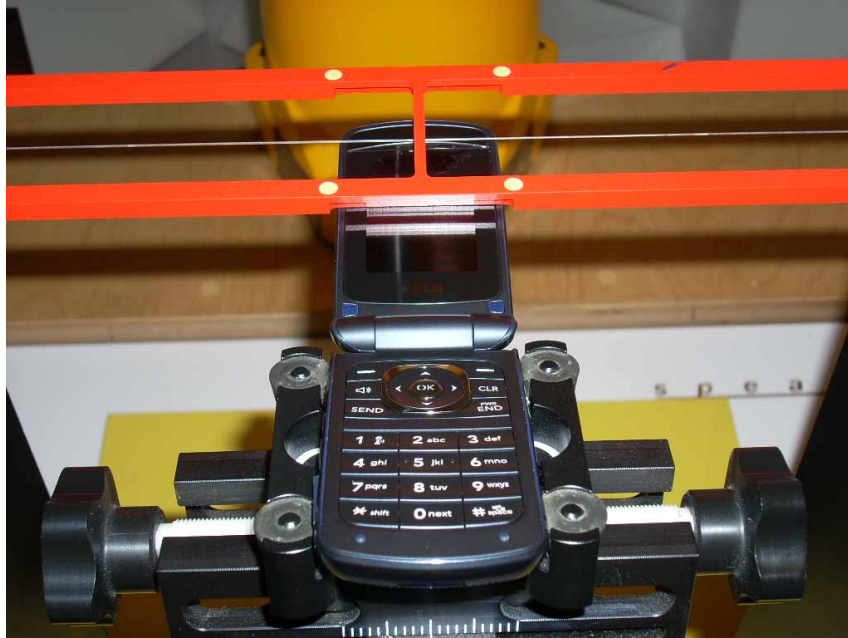
Figure 17-1 Ear Reference Point HAC Phantom Alignment
