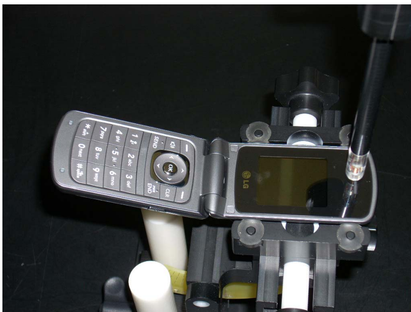
Figure 13-1 Test Setup for Wireless Device
