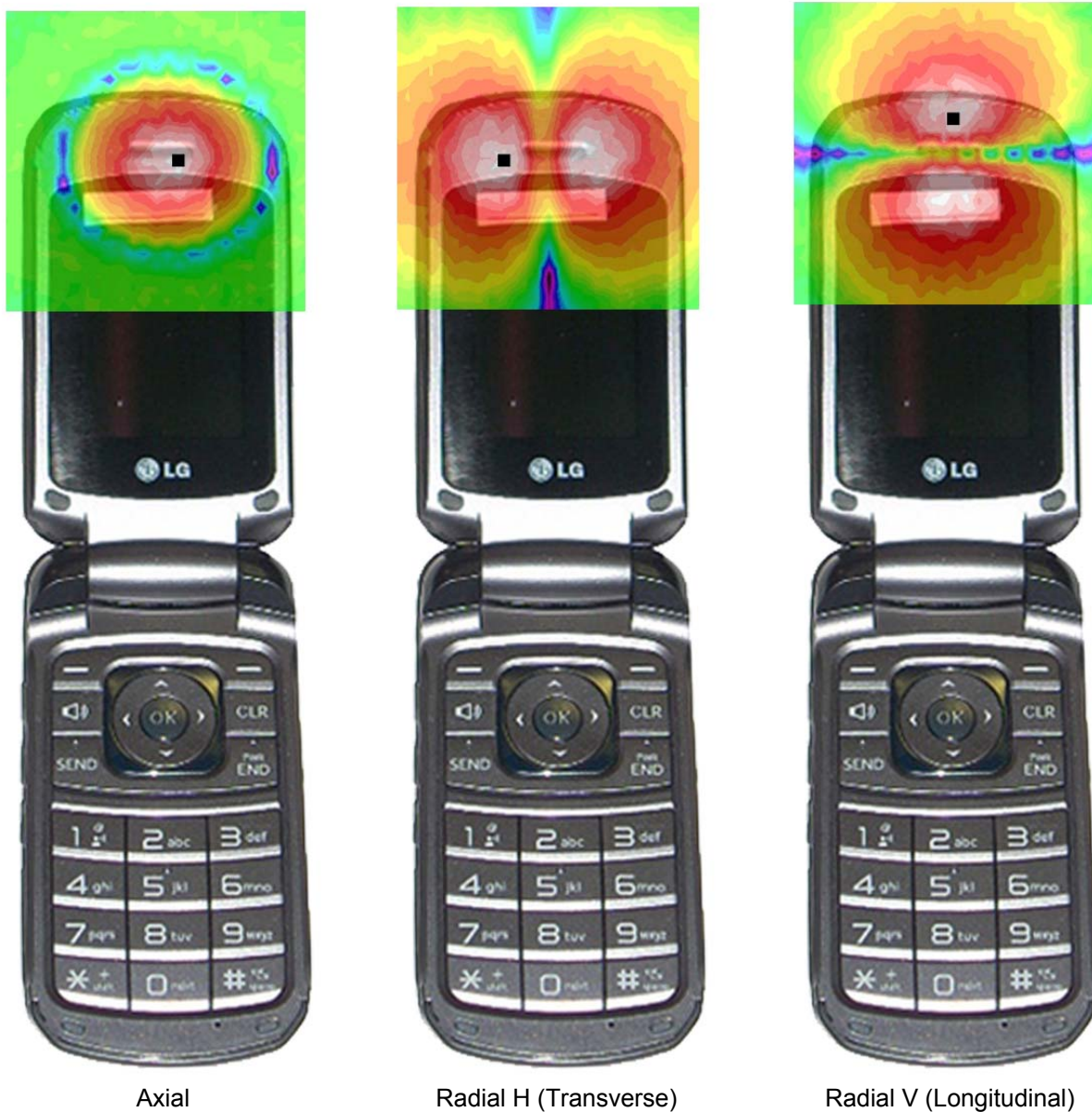
Figure 13-3 T-Coil Scan Overlay Magnetic Field Distributions
