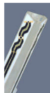
Figure 3.2 Probe Thick-Film Technique
