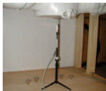
Figure 12.1 Dipole Validation Test Setup
