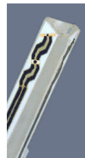
Figure 3.2 Probe Thick-Film Technique
