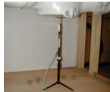
Figure 12.1 Dipole Validation Test Setup
