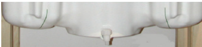
Figure 7.2 SAM Twin Phantom shell
