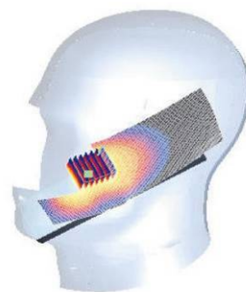
Figure 7-1 Sample SAR Area Scan
