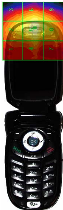
Figure 30 E-Field WD Scan overlay
