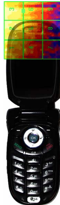
Figure 31 H-Field WD Scan overlay
