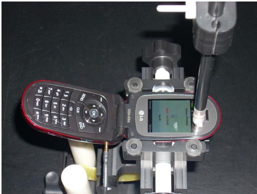
Figure 13-1 Test Setup for Wireless Device
