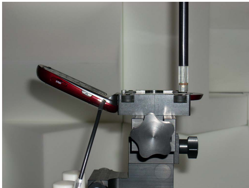
Figure 13-2 Test Setup for Wireless Device
