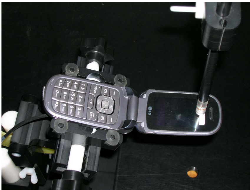
Figure 13-2 Test Setup for Wireless Device
