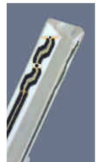
Figure 3.2 Probe Thick-Film Technique
