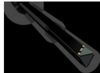
Figure 4-3 Triangular Probe Configuration
