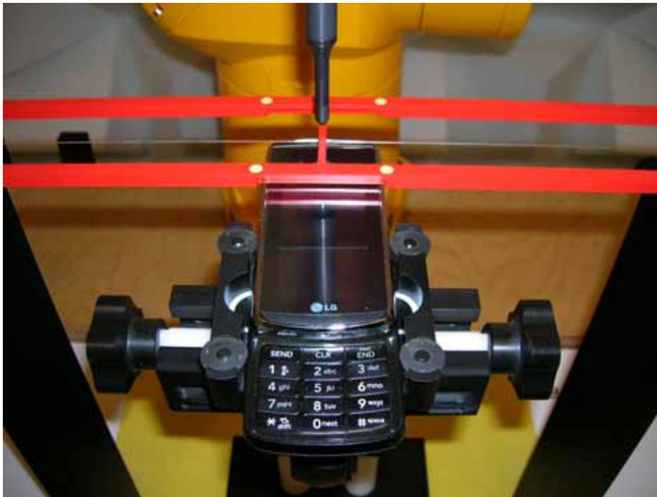
Figure 17-2 HAC Phantom Plane Alignment
