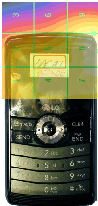
Figure 17-4 E-Field WD Scan overlay
