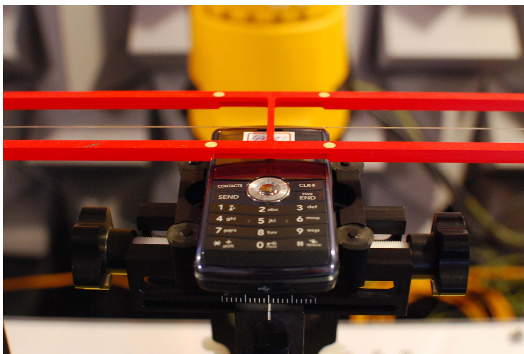
Figure 17-2 HAC Phantom Plane Alignment
