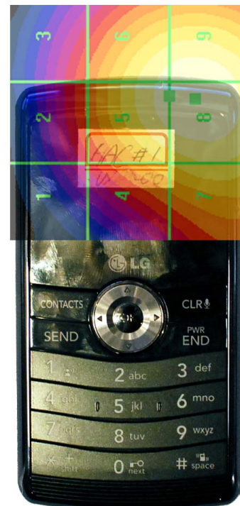
Figure 17-5 H-Field WD Scan overlay
