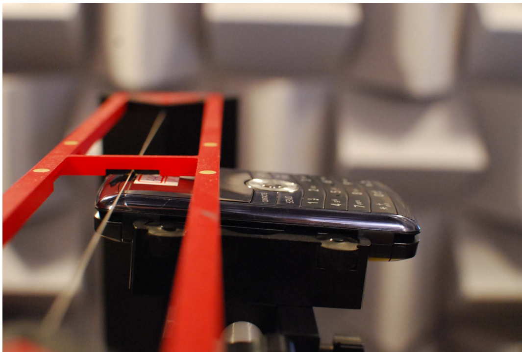
Figure 17-1 Ear Reference Point HAC Phantom Alignment
