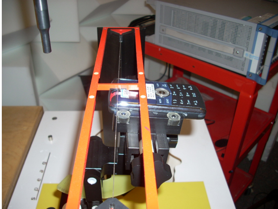
Figure 17-1 Ear Reference Point HAC Phantom Alignment
