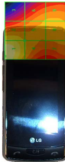
Figure 17-7 H-Field WD Scan overlay
