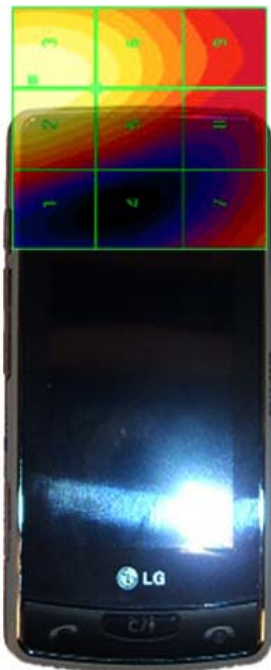
Figure 17-6 E-Field WD Scan overlay
