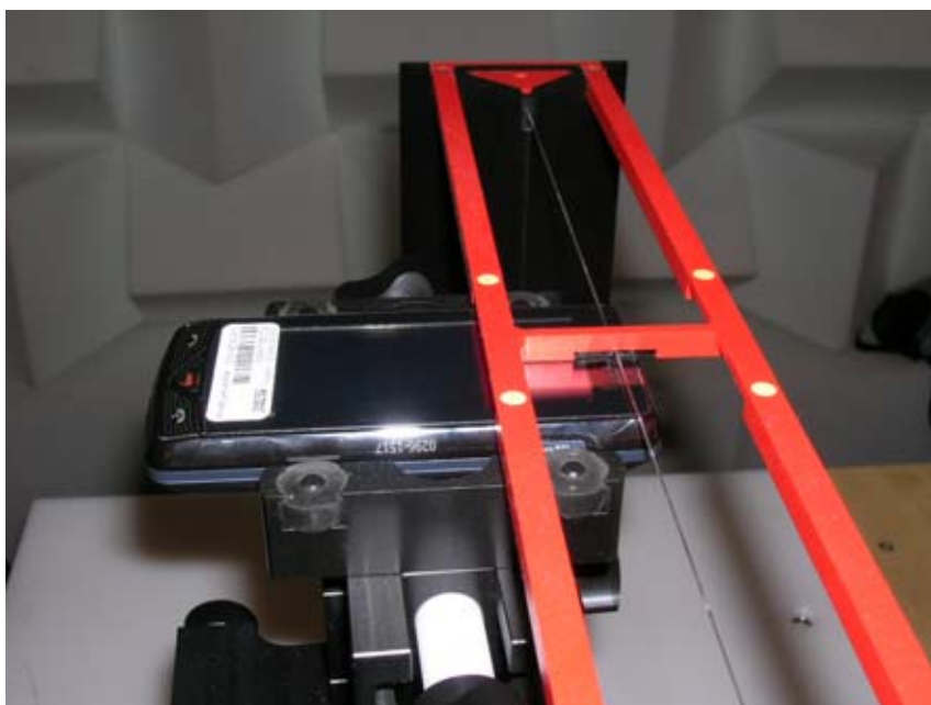
Figure 17-2 HAC Phantom Plane Alignment
