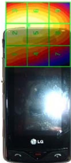
Figure 17-4 E-Field WD Scan overlay
