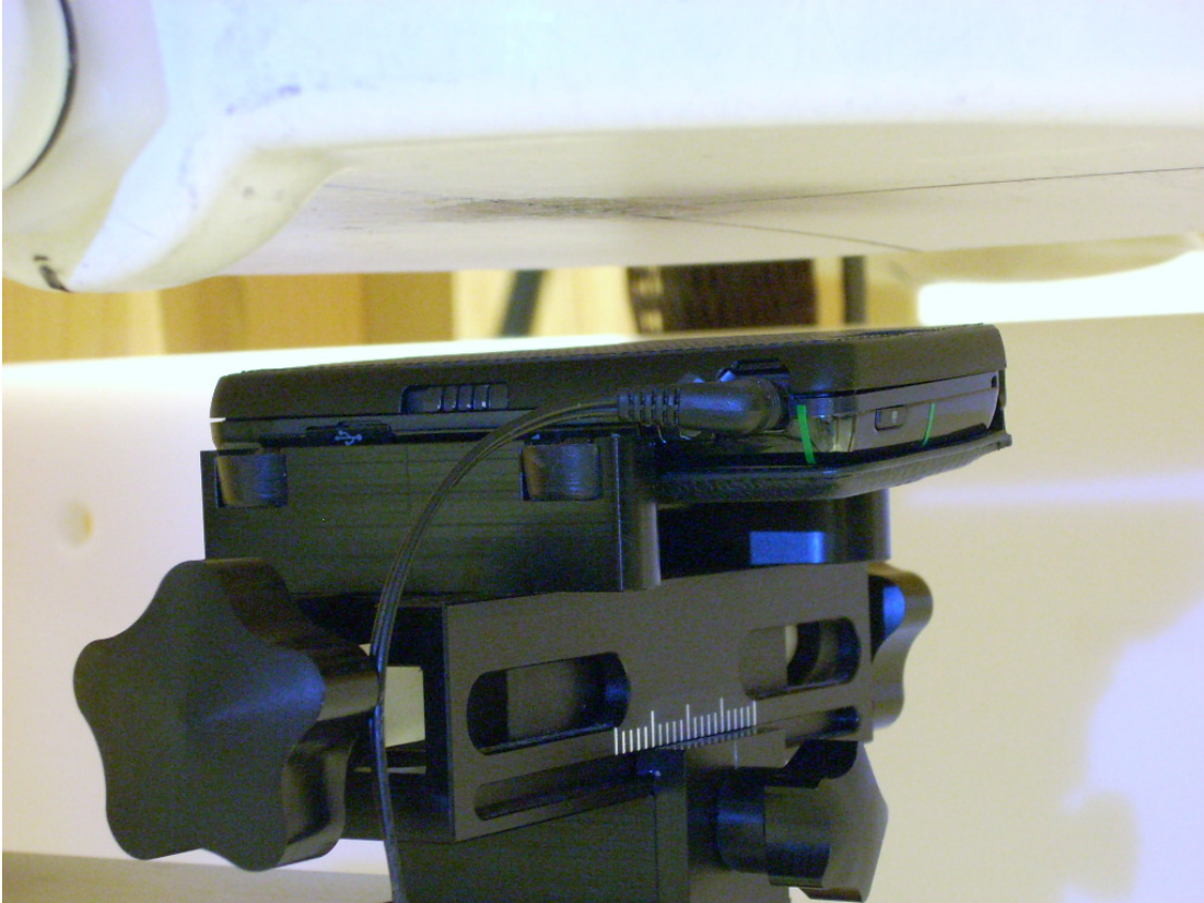
11. Body SAR, Back Side with Keyboard 20mm Space
