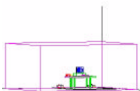
Figure 3-1. Shielded Enclosure Line-Conducted Test Facility
