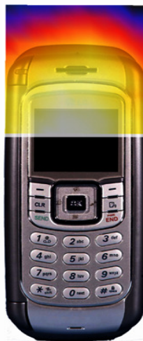
Figure 28 Sample H-field Scan Overlay
