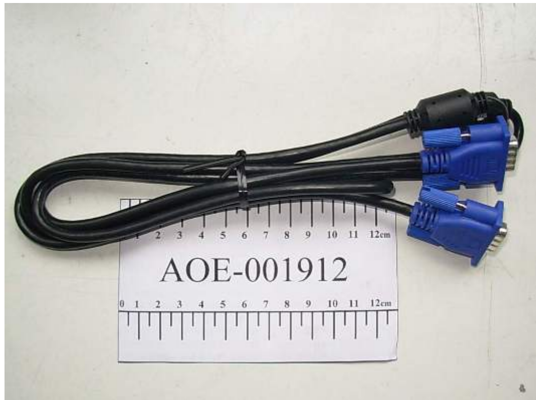
FIGURE 5 LCD MONITOR (M/N: W1542ST) D-SUB CABLE
