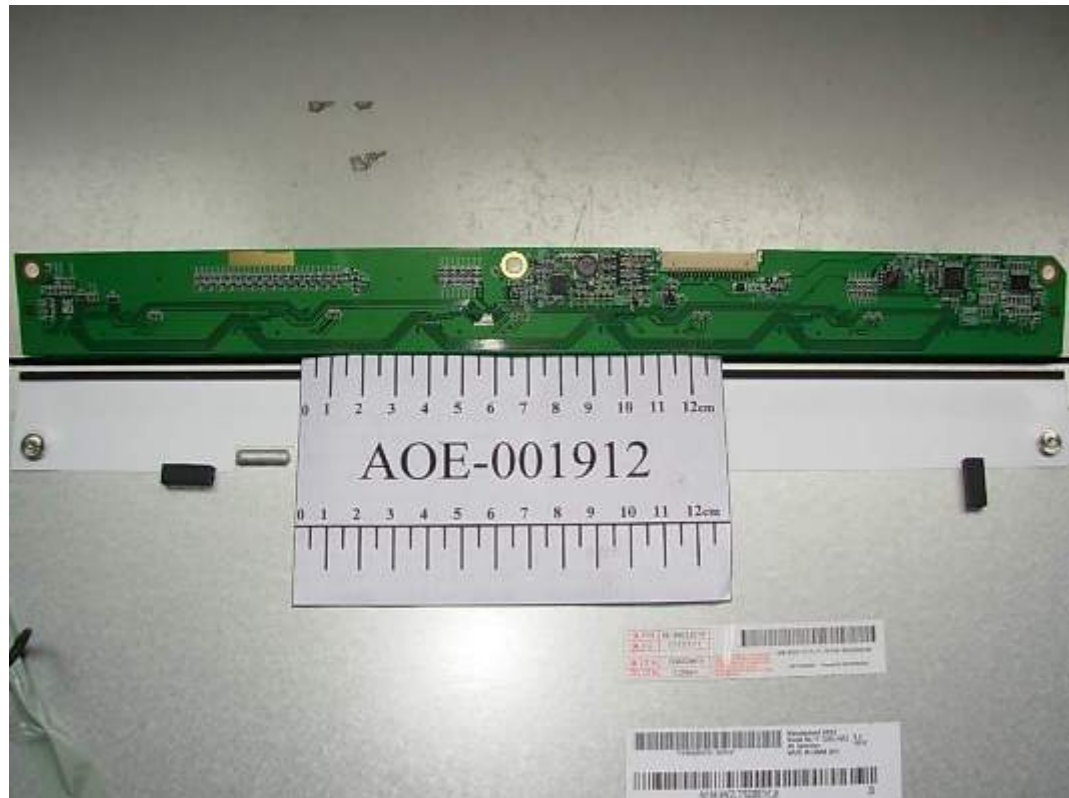
FIGURE 12 LCD MONITOR (M/N: W1542ST) LCD PANEL MAIN BOARD (COMPONENT SIDE)
