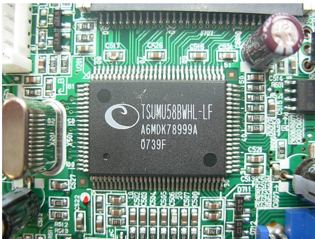
FIGURE 10 LCD MONITOR (M/N: W1752ST) CHIP ON MAIN BOARD
