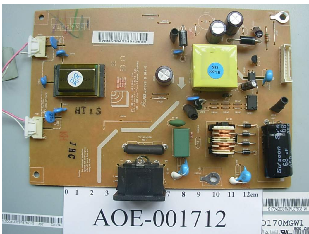
FIGURE 11 LCD MONITOR (M/N: W1752ST) POWER BOARD (FRONT VIEW)
