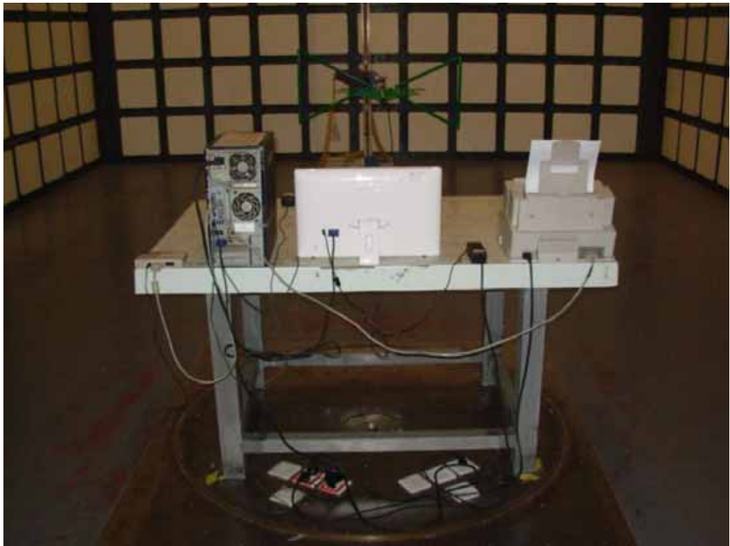
BACK VIEW OF RADIATED EMISSION TEST
