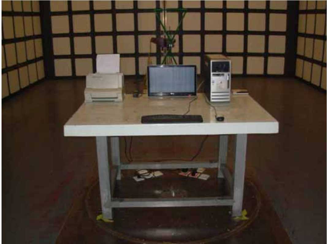
FRONT VIEW OF RADIATED EMISSION TEST
