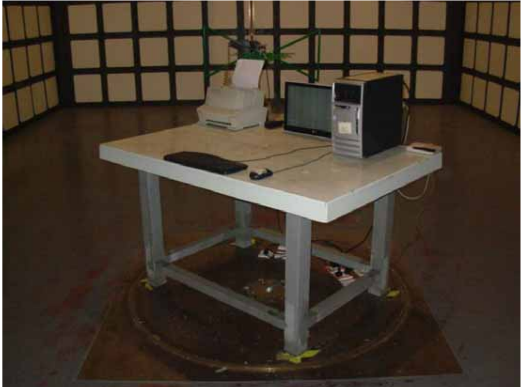
SETUP WITH MAXIMUM DETECTED EMISSION AT HORIZONTAL POLARIZATION (TEST MODE: D-SUB 1024*768@60Hz, ADAPTER: ADS-24NP-12-1 12024G)
