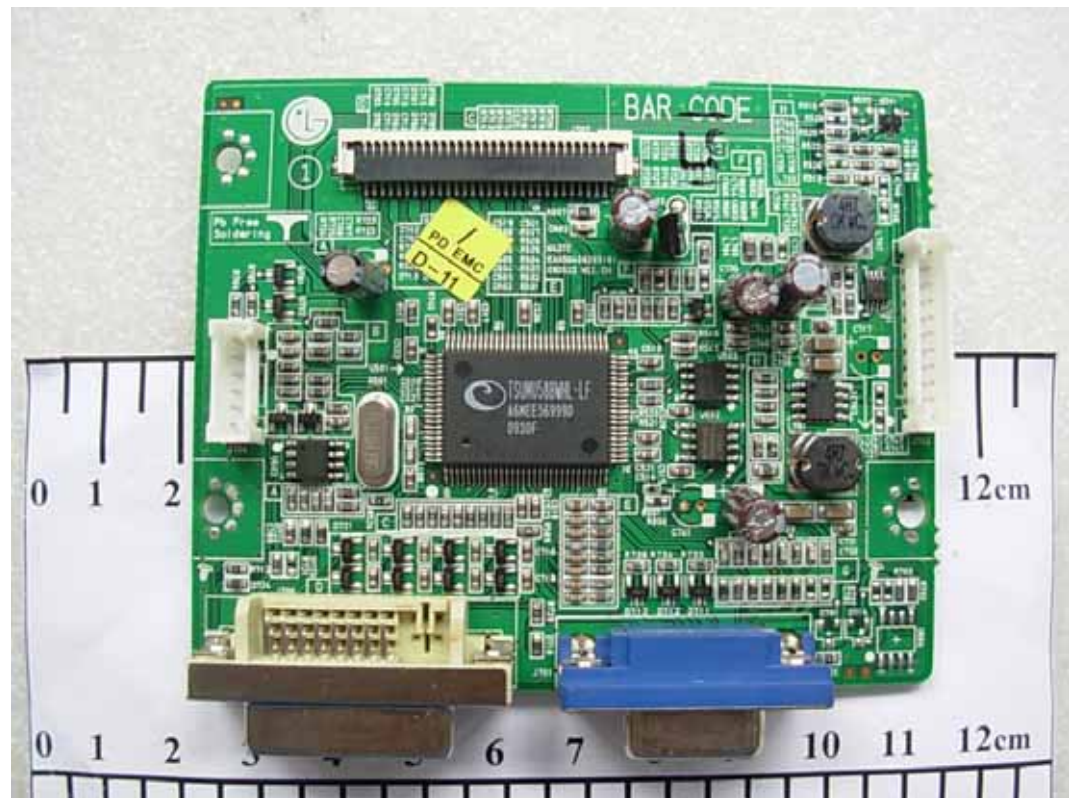
FIGURE 2 LCD MONITOR (M/N: W1942PEU) MAIN BOARD (COMPONENT SIDE)
