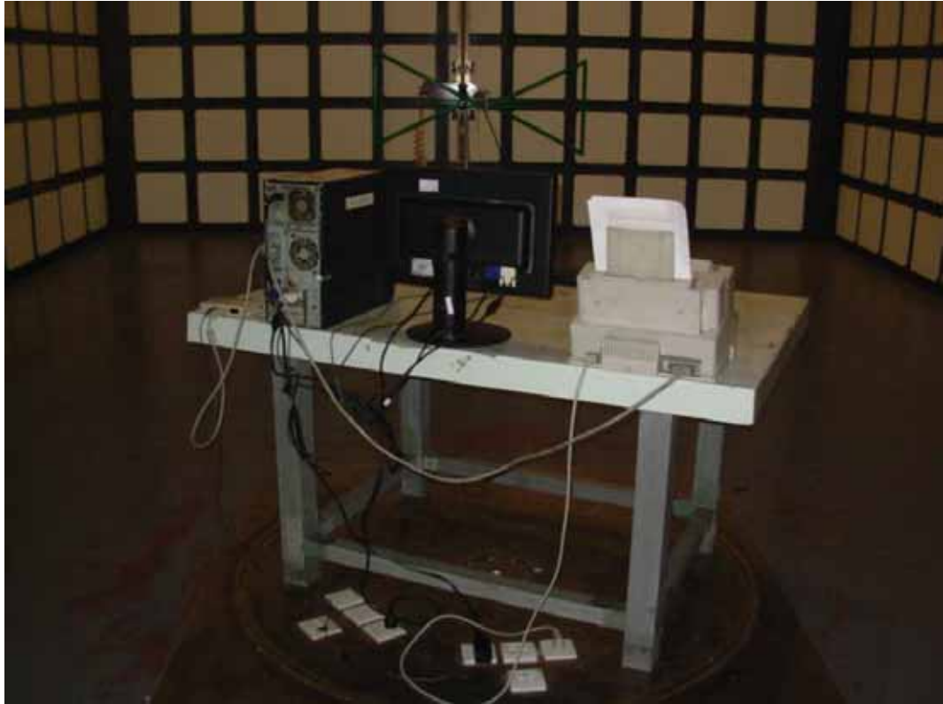
SETUP WITH MAXIMUM DETECTED EMISSION AT HORIZONTAL POLARIZATION (M/N: W1942PEU, TEST MODE: DVI 1280*1024@75Hz)
