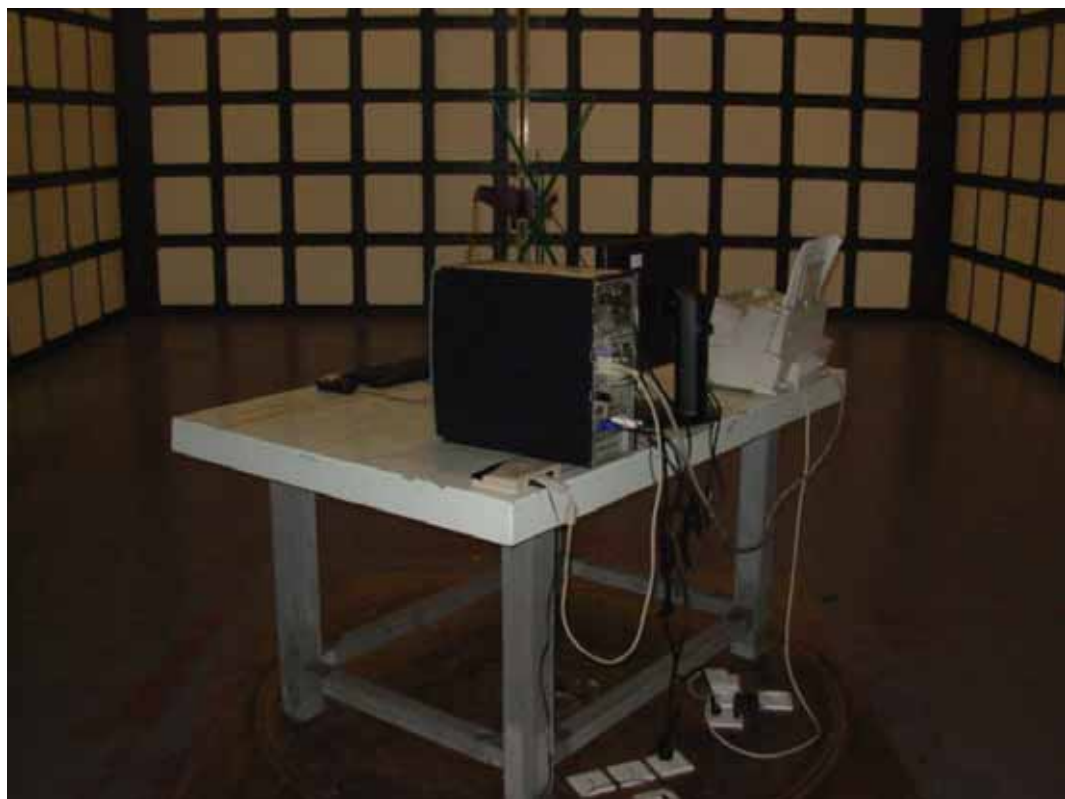
SETUP WITH MAXIMUM DETECTED EMISSION AT VERTICAL POLARIZATION (M/N: W1942PEU, TEST MODE: DVI 1280*1024@75Hz)
