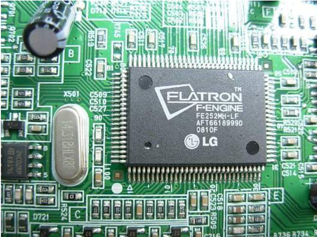
FIGURE 7 LCD MONITOR (M/N: W1942TET) CHIP & CRYSTAL ON MAIN BOARD (SOLDERED SIDE)
