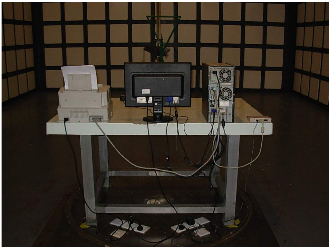
BACK VIEW OF RADIATED EMISSION TEST
