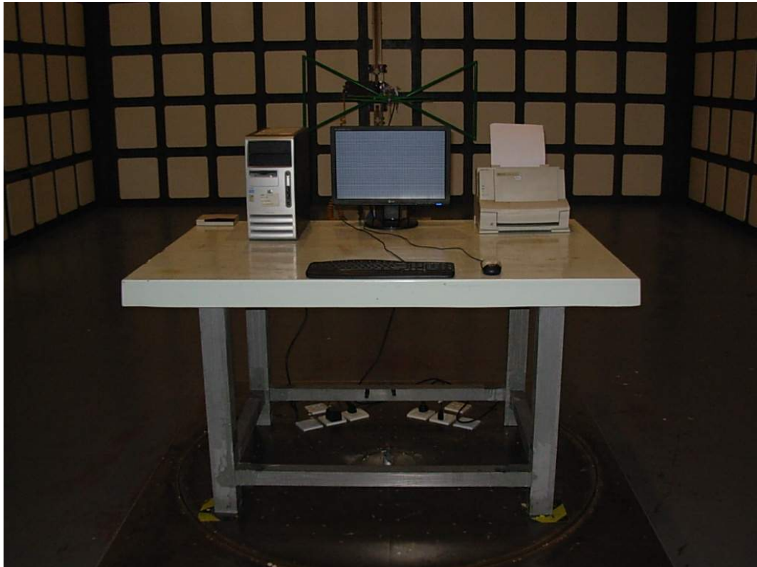
FRONT VIEW OF RADIATED EMISSION TEST
