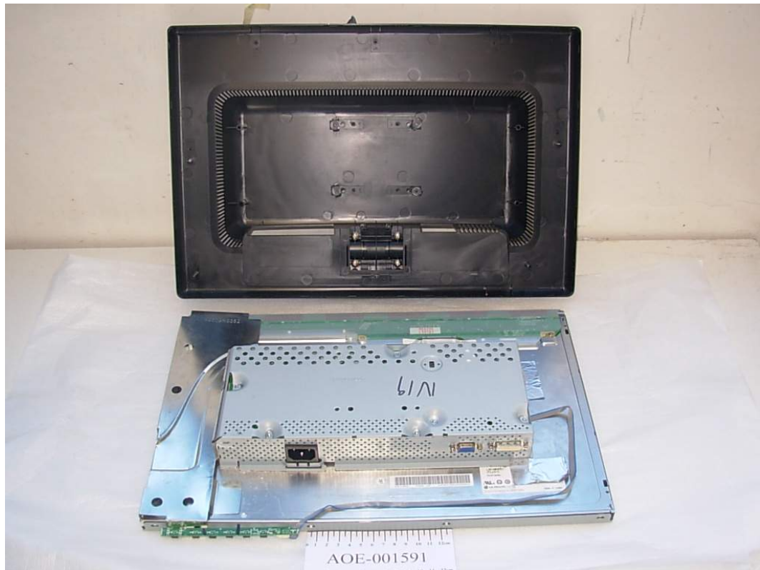
FIGURE 1 LCD MONITOR (M/N: W1942TT) COVER REMOVED
