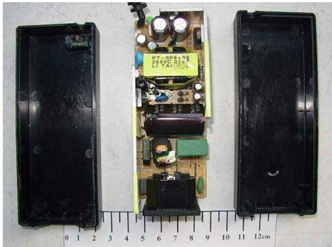
FIGURE 16 LCD MONITOR (M/N: W1943CMV) ADAPTOR COVER REMOVED
