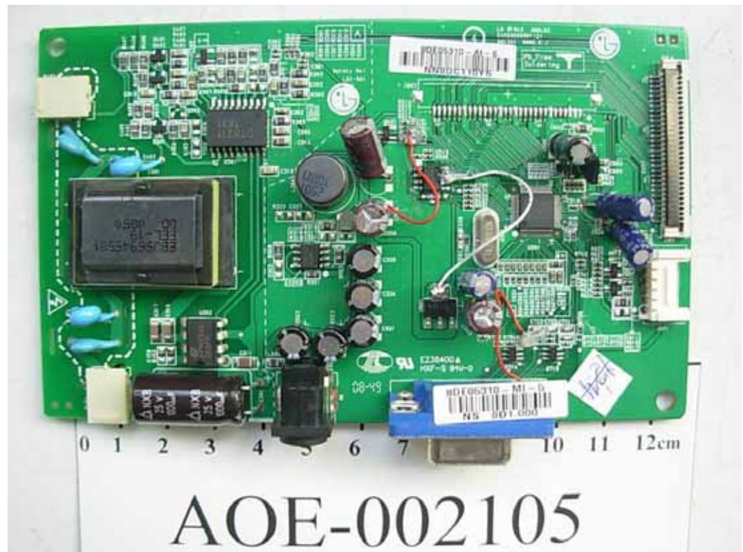
FIGURE 5 LCD MONITOR (M/N: W1943SV) MAIN BOARD (COMPONENT SIDE)
