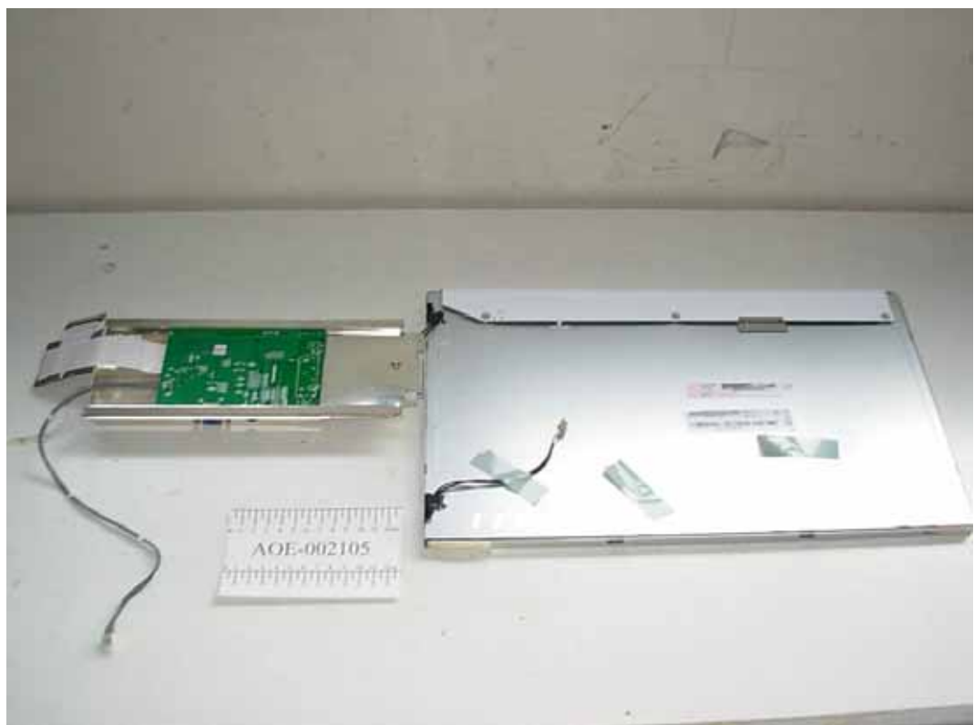
FIGURE 2 LCD MONITOR (M/N: W1943SV) BOARDS REMOVED
