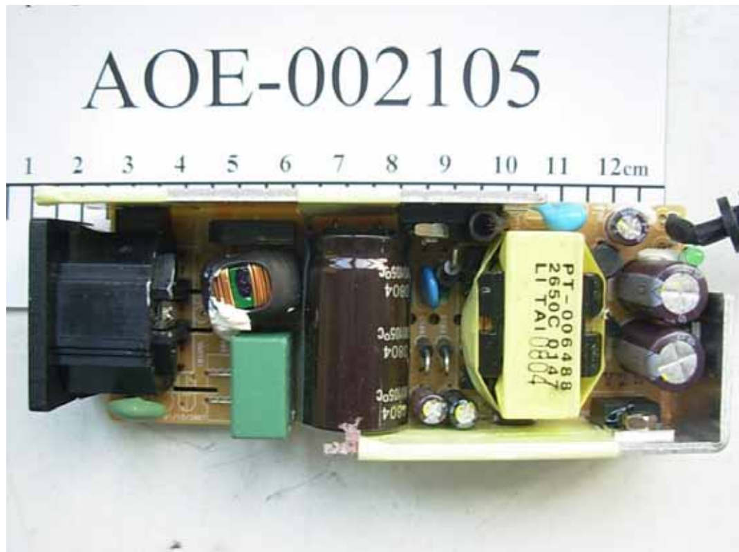
FIGURE 35 LCD MONITOR (M/N: W1943SV, W1943CV) ADAPTOR #1 MAIN BOARD (COMPONENT SIDE)
