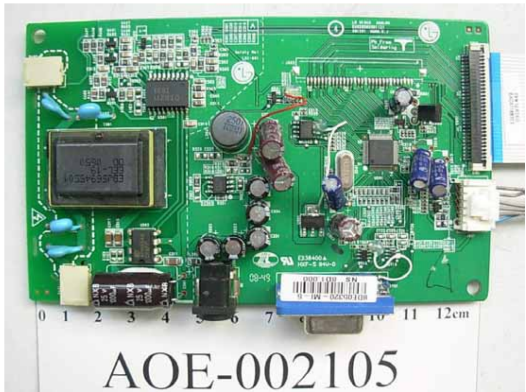
FIGURE 19 LCD MONITOR (M/N: W1943CV) MAIN BOARD (COMPONENT SIDE)
