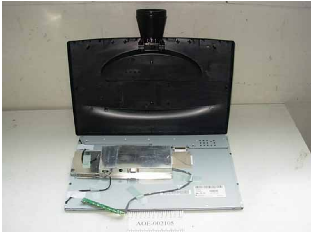
FIGURE 15 LCD MONITOR (M/N: W1943CV) COVER REMOVED
