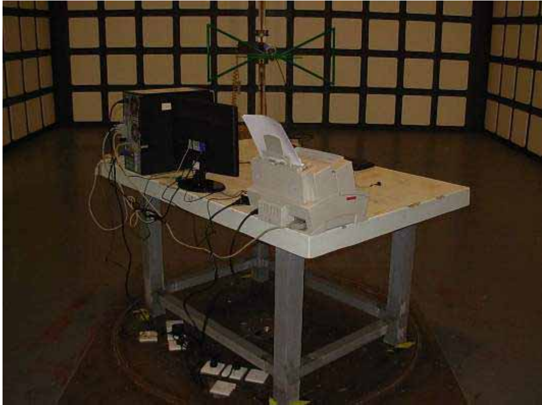
SETUP WITH MAXIMUM DETECTED EMISSION AT HORIZONTAL POLARIZATION (D-SUB 640*480@60Hz)
