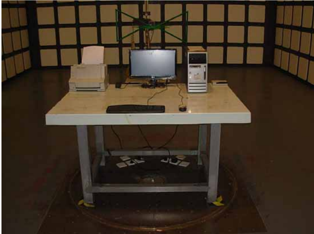
FRONT VIEW OF RADIATED EMISSION TEST (ADAPTOR: LCAP07F)
