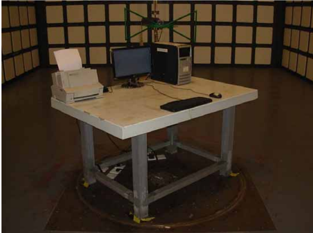
SETUP WITH MAXIMUM DETECTED EMISSION AT HORIZONTAL POLARIZATION (M/N: W1943SV, TEST MODE: D-SUB 1360*768@60Hz) (ADAPTOR: LCAP07F)
