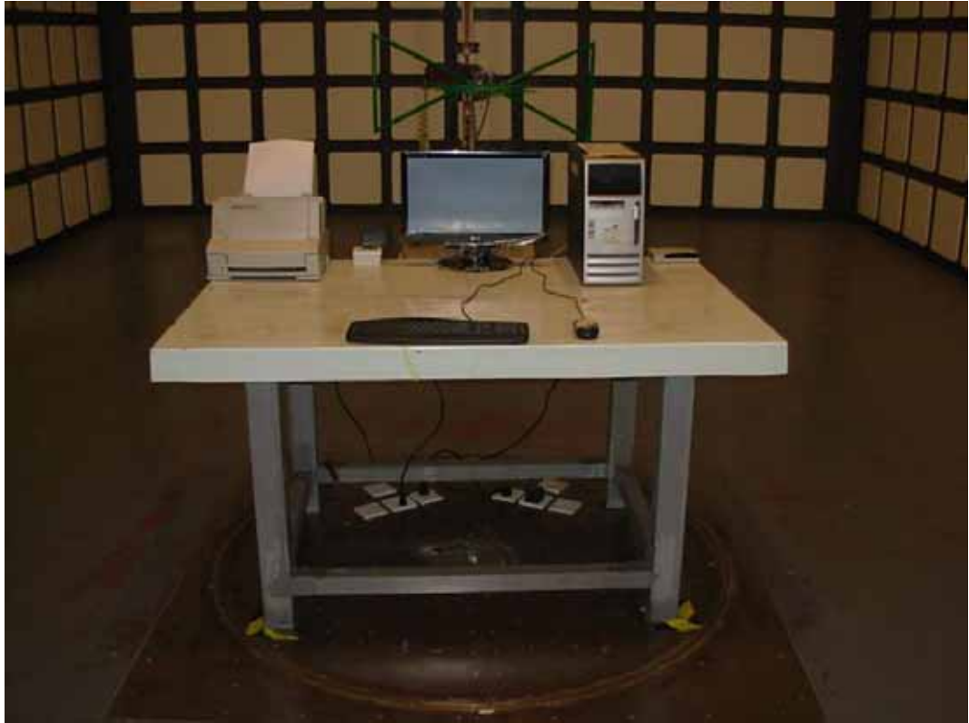
FRONT VIEW OF RADIATED EMISSION TEST (ADAPTOR: ADS-24S-12 1224GPCN)
