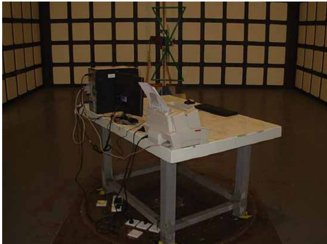
SETUP WITH MAXIMUM DETECTED EMISSION AT VERTICAL POLARIZATION (M/N: W1943SV, TEST MODE: D-SUB 1360*768@60Hz) (ADAPTOR: LCAP07F)
