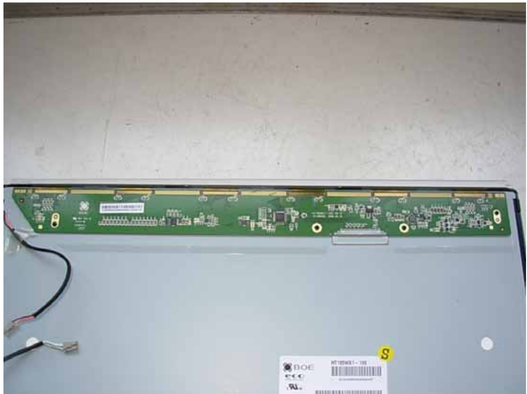
FIGURE 9 LCD MONITOR (M/N: W1946SW) LCD PANEL BOARD (COMPONENT SIDE)
