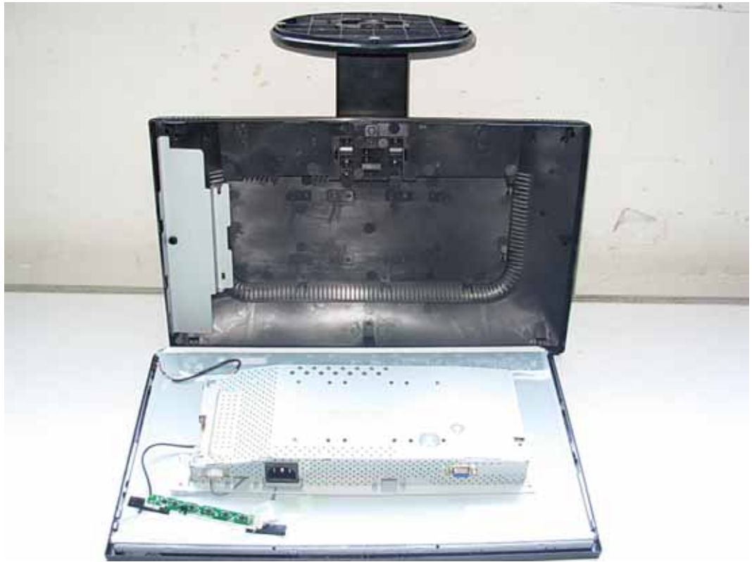
FIGURE 1 LCD MONITOR (M/N: W1946SW) COVER REMOVED
