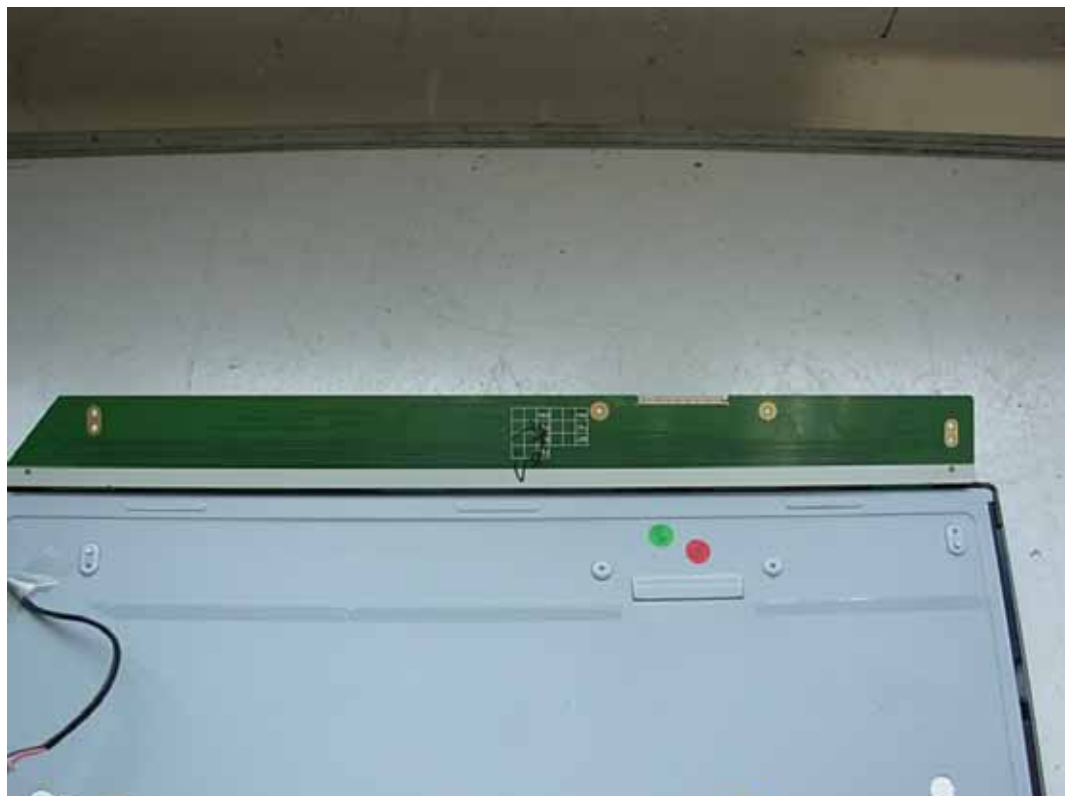
FIGURE 10 LCD MONITOR (M/N: W1946SW) LCD PANEL BOARD (SOLDERED SIDE)
