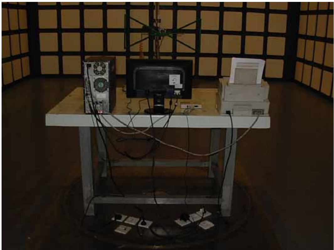
BACK VIEW OF RADIATED EMISSION TEST
