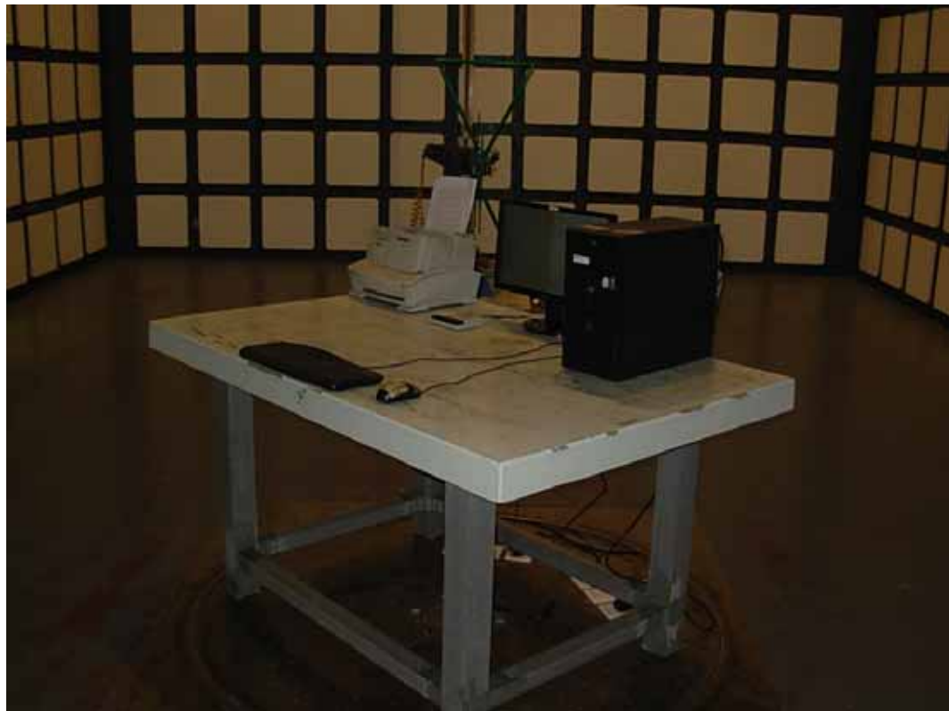
SETUP WITH MAXIMUM DETECTED EMISSION AT VERTICAL POLARIZATION (TEST MODE: DVI 1024*768@60Hz)
