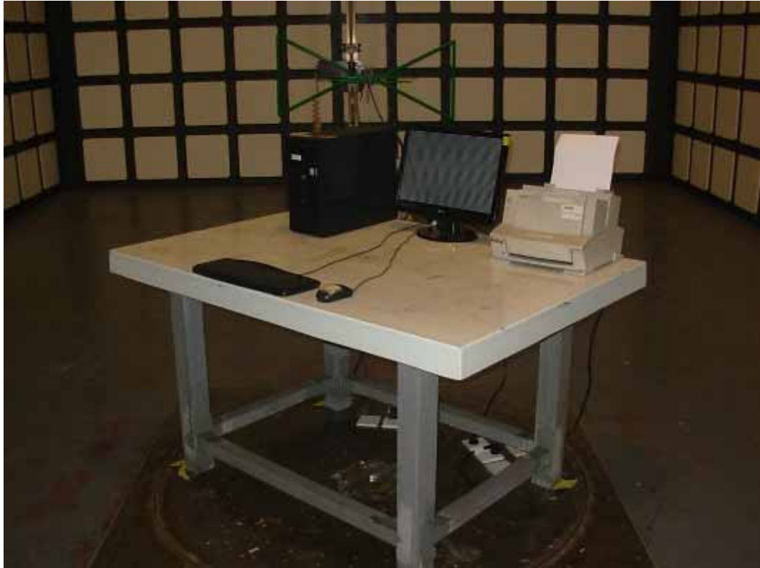
SETUP WITH MAXIMUM DETECTED EMISSION AT HORIZONTAL POLARIZATION (D-SUB 1440*900@75Hz)
