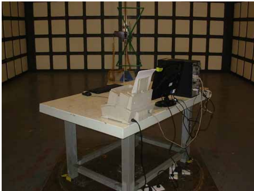
SETUP WITH MAXIMUM DETECTED EMISSION AT VERTICAL POLARIZATION (D-SUB 1440*900@75Hz)
