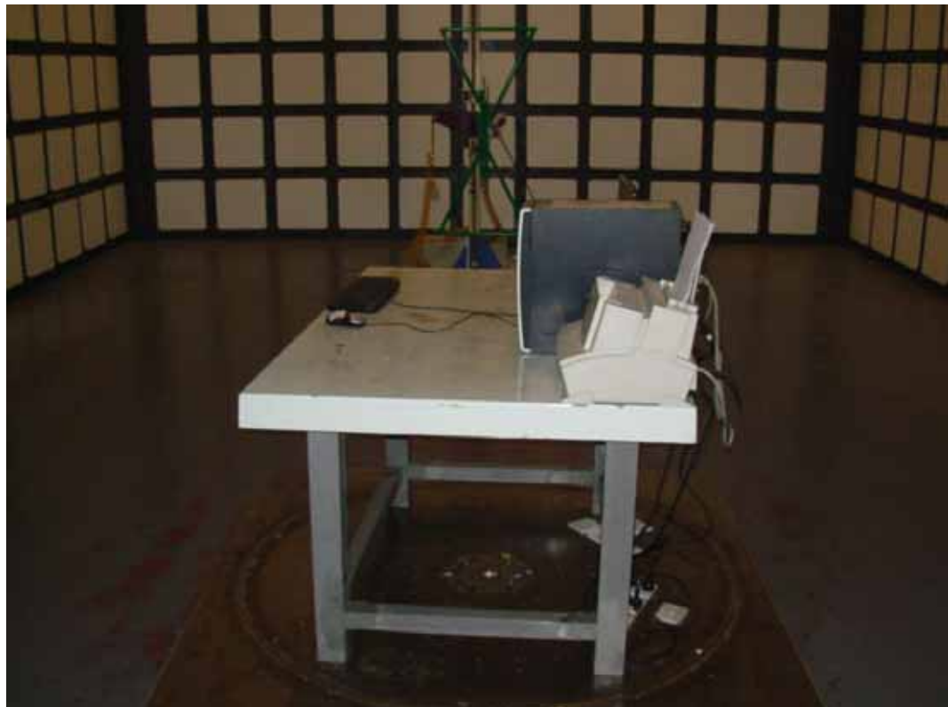
SETUP WITH MAXIMUM DETECTED EMISSION AT VERTICAL POLARIZATION (DVI 1600*900@60Hz)
