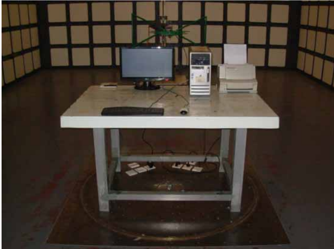
FRONT VIEW OF RADIATED EMISSION TEST
