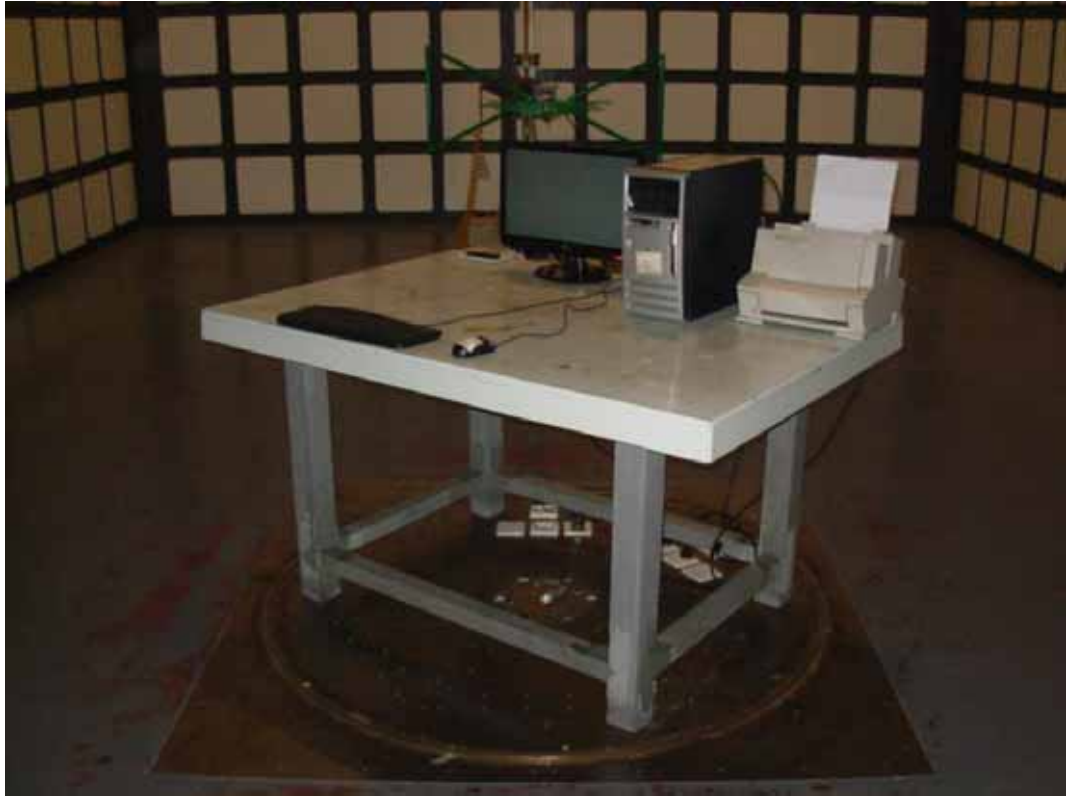
SETUP WITH MAXIMUM DETECTED EMISSION AT HORIZONTAL POLARIZATION (DVI 1600*900@60Hz)
