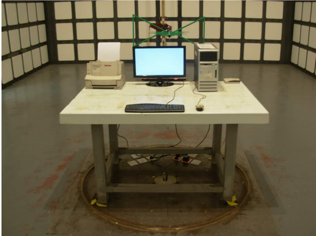
FRONT VIEW OF RADIATED EMISSION TEST
