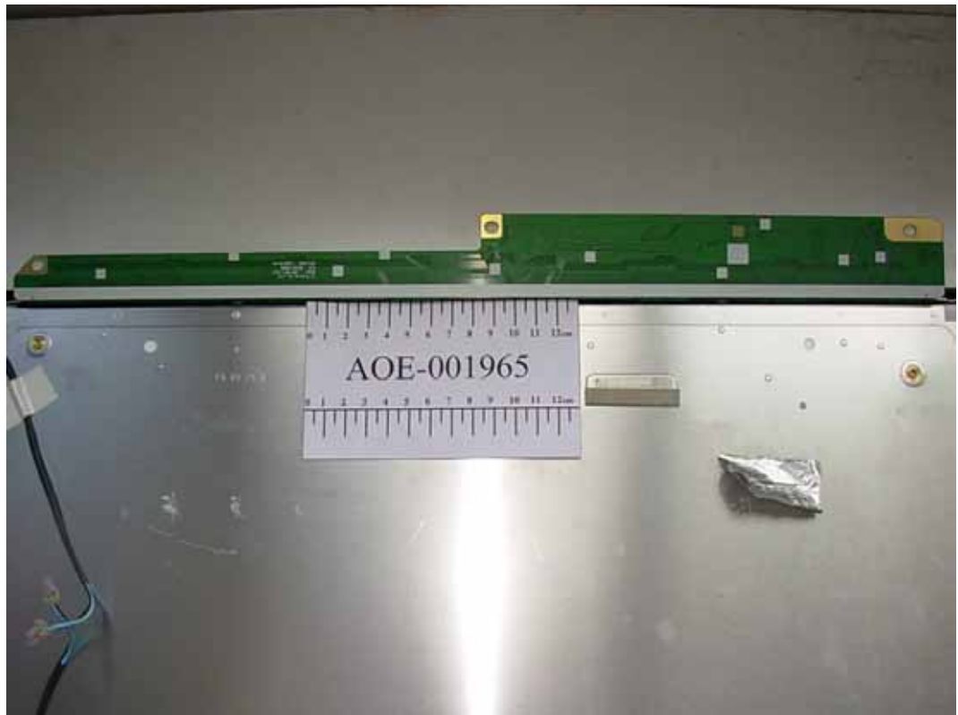
FIGURE 13 LCD MONITOR (M/N: W2242TET) LCD PANEL MAIN BOARD (SOLDERED SIDE)
