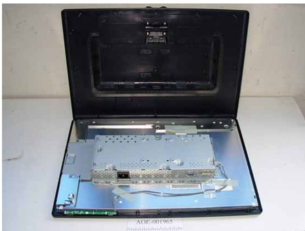
FIGURE 1 LCD MONITOR (M/N: W2242TET) COVER REMOVED
