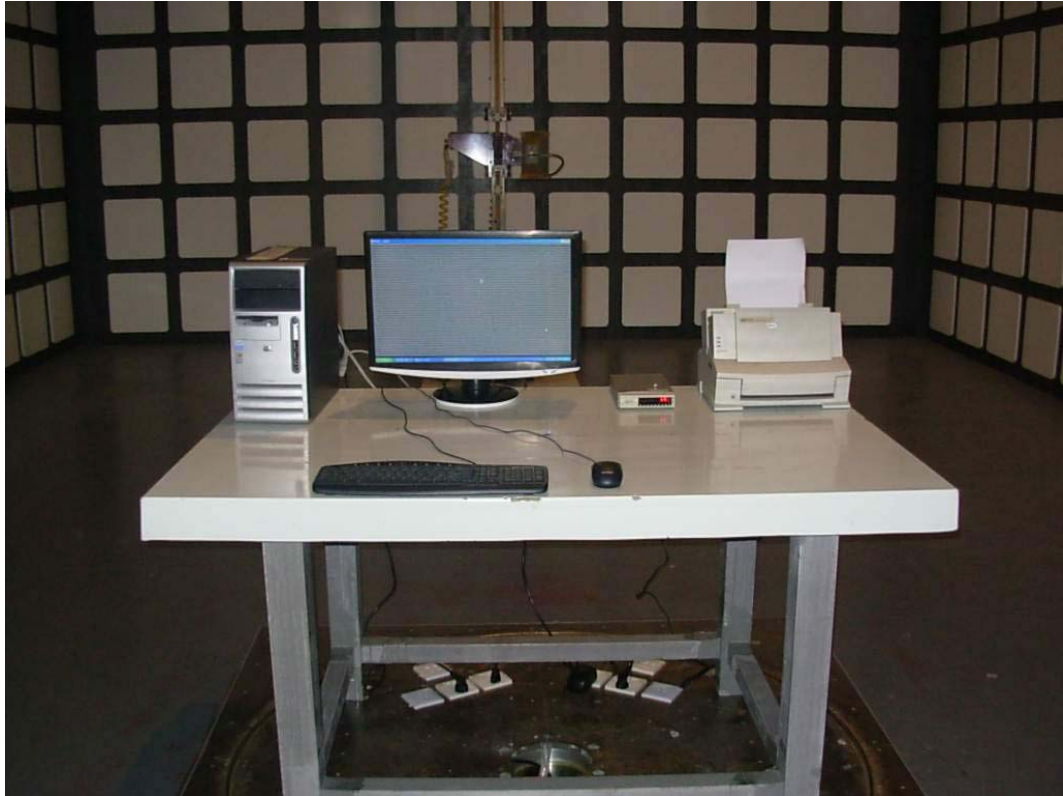
FRONT VIEW OF RADIATED EMISSION TEST (HIGH FREQUENCY)
