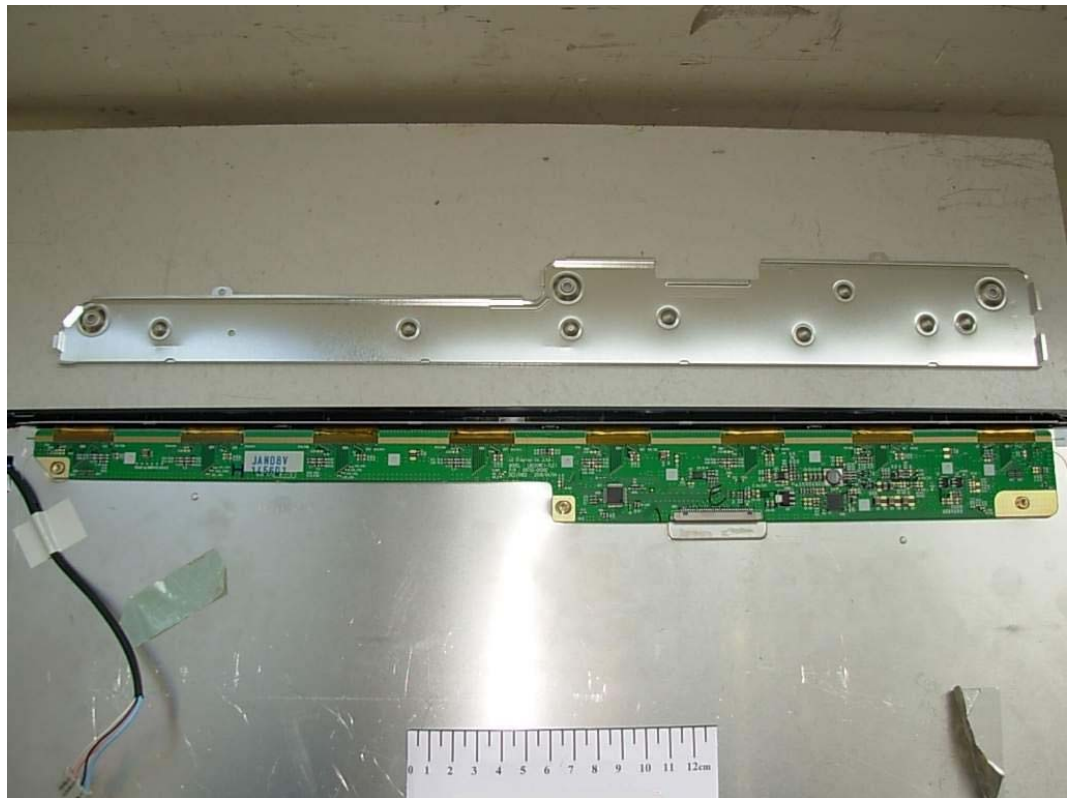
FIGURE 12 LCD MONITOR (M/N: W2254VQV) LCD PANEL MAIN BOARD (COMPONENT SIDE)
