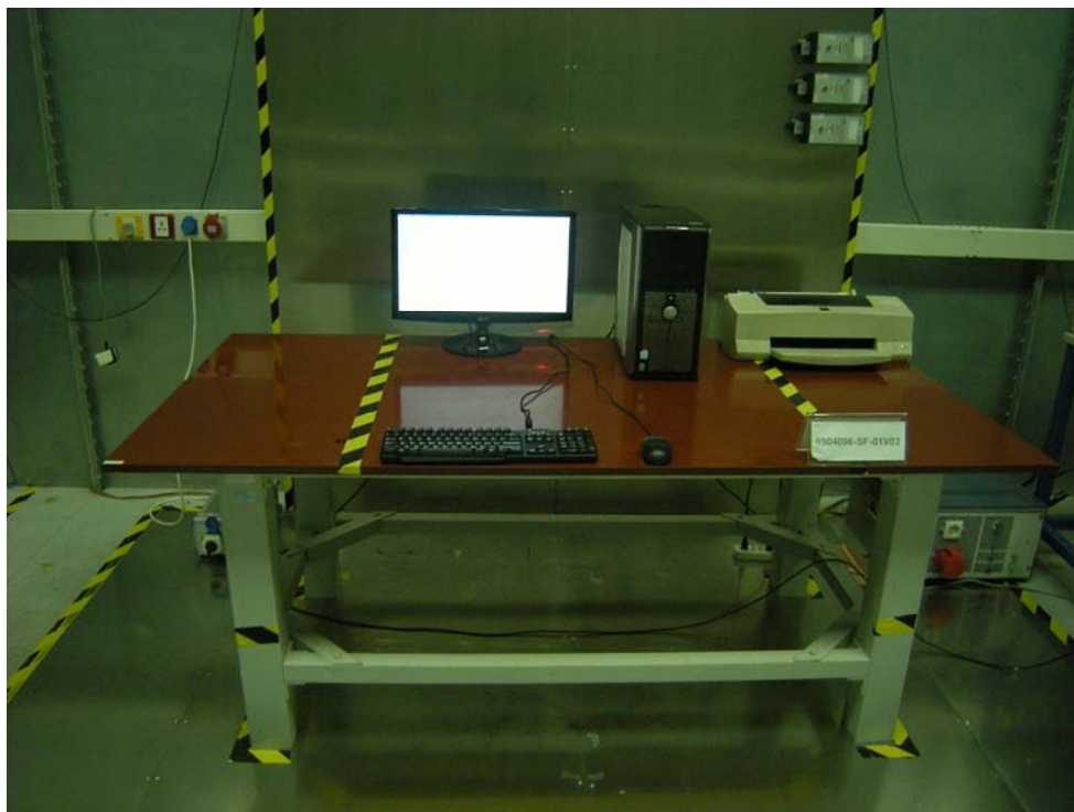
Front View of Conducted Emission Test
