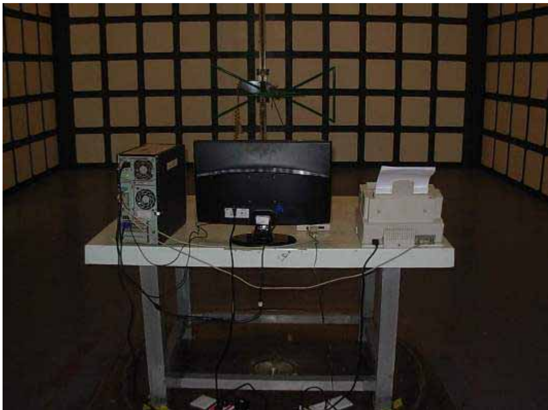
BACK VIEW OF RADIATED EMISSION TEST
