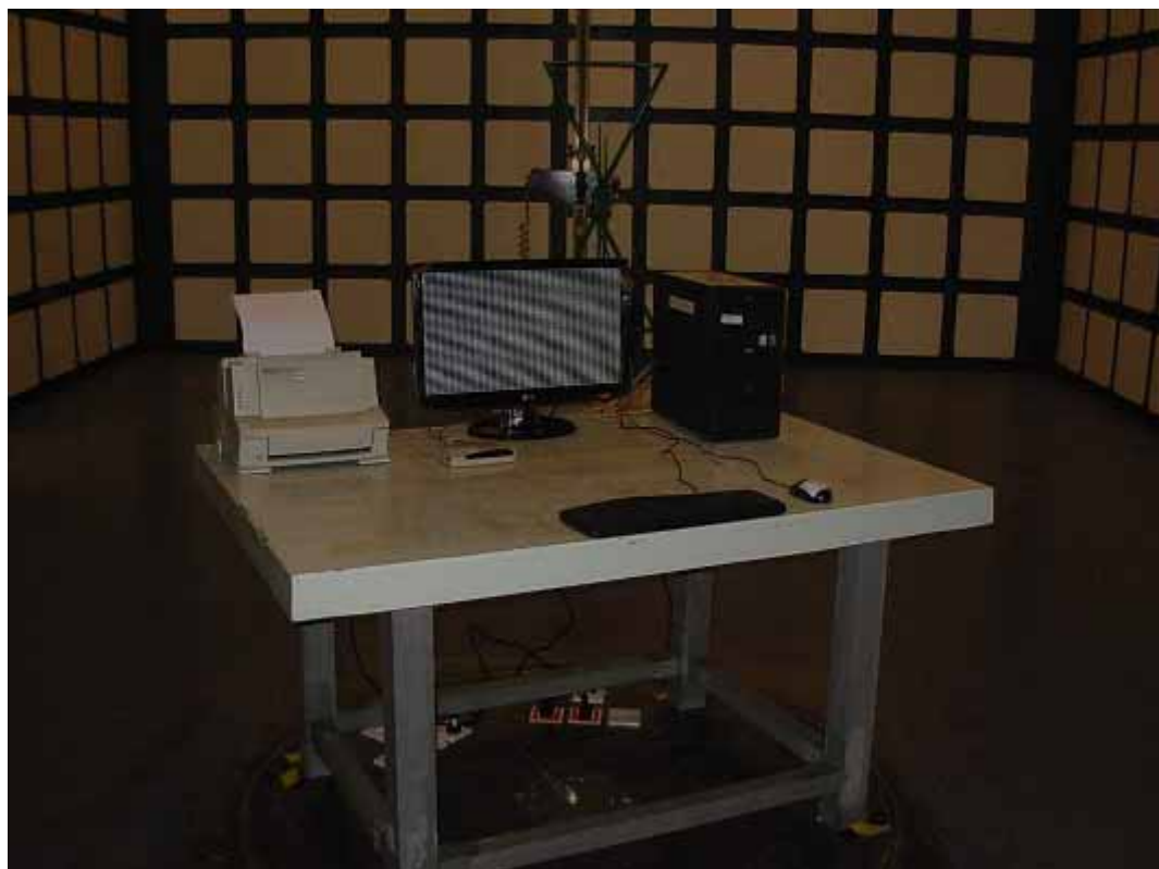
SETUP WITH MAXIMUM DETECTED EMISSION AT VERTICAL POLARIZATION (D-SUB 640*480@60Hz)
