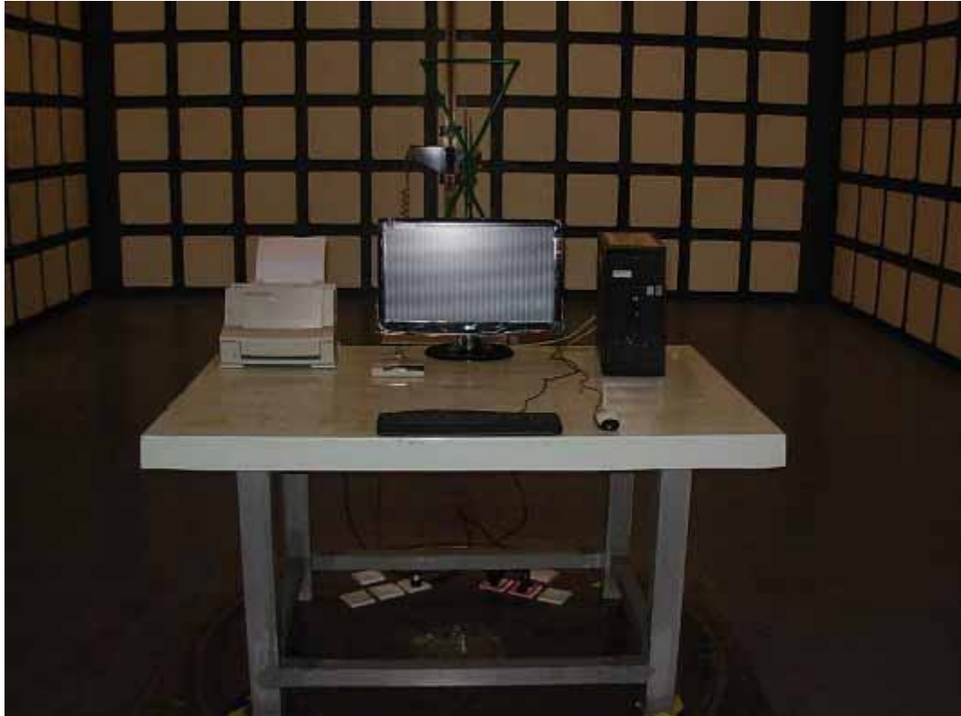
FRONT VIEW OF RADIATED EMISSION TEST
