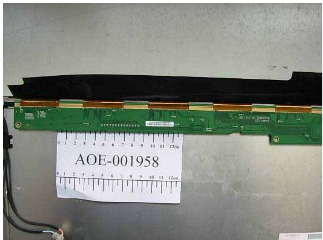
FIGURE 16 LCD MONITOR (M/N: W2442PAT) LCD PANEL MAIN BOARD (SOLDERED SIDE) 2
