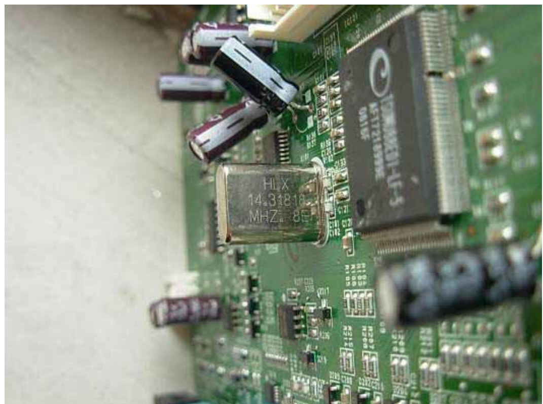
FIGURE 10 LCD MONITOR (M/N: W2442PAT) CRYSTAL ON MAIN BOARD
