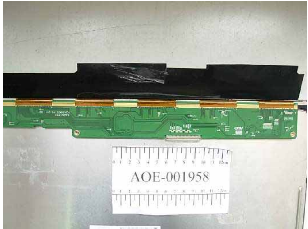
FIGURE 15 LCD MONITOR (M/N: W2442PAT) LCD PANEL MAIN BOARD (SOLDERED SIDE) 1
