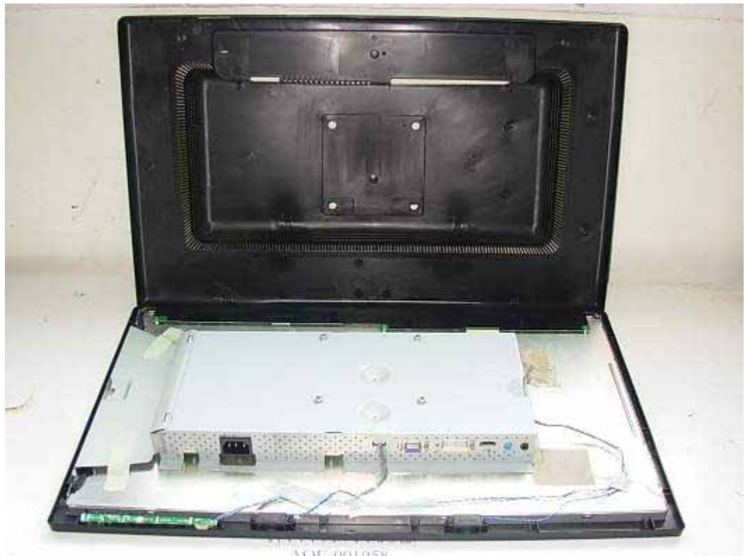
FIGURE 1 LCD MONITOR (M/N: W2442PAT) COVER REMOVED
