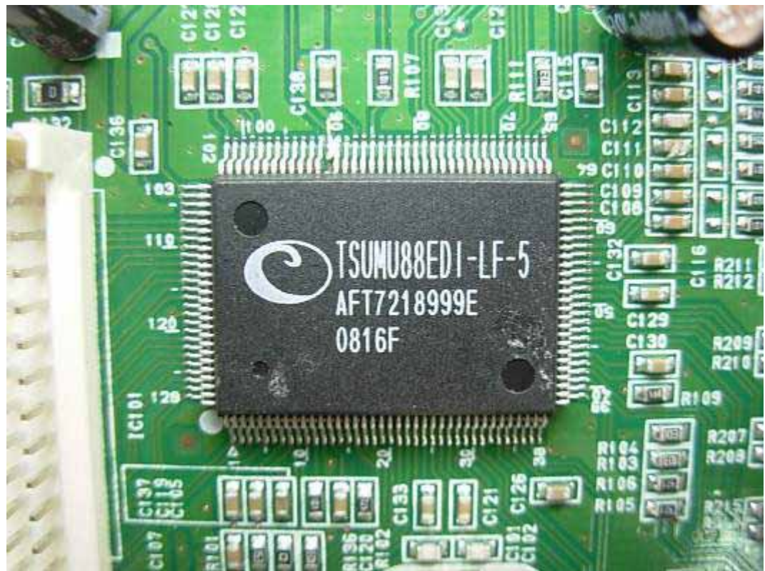
FIGURE 9 LCD MONITOR (M/N: W2442PAT) CHIP ON MAIN BOARD
