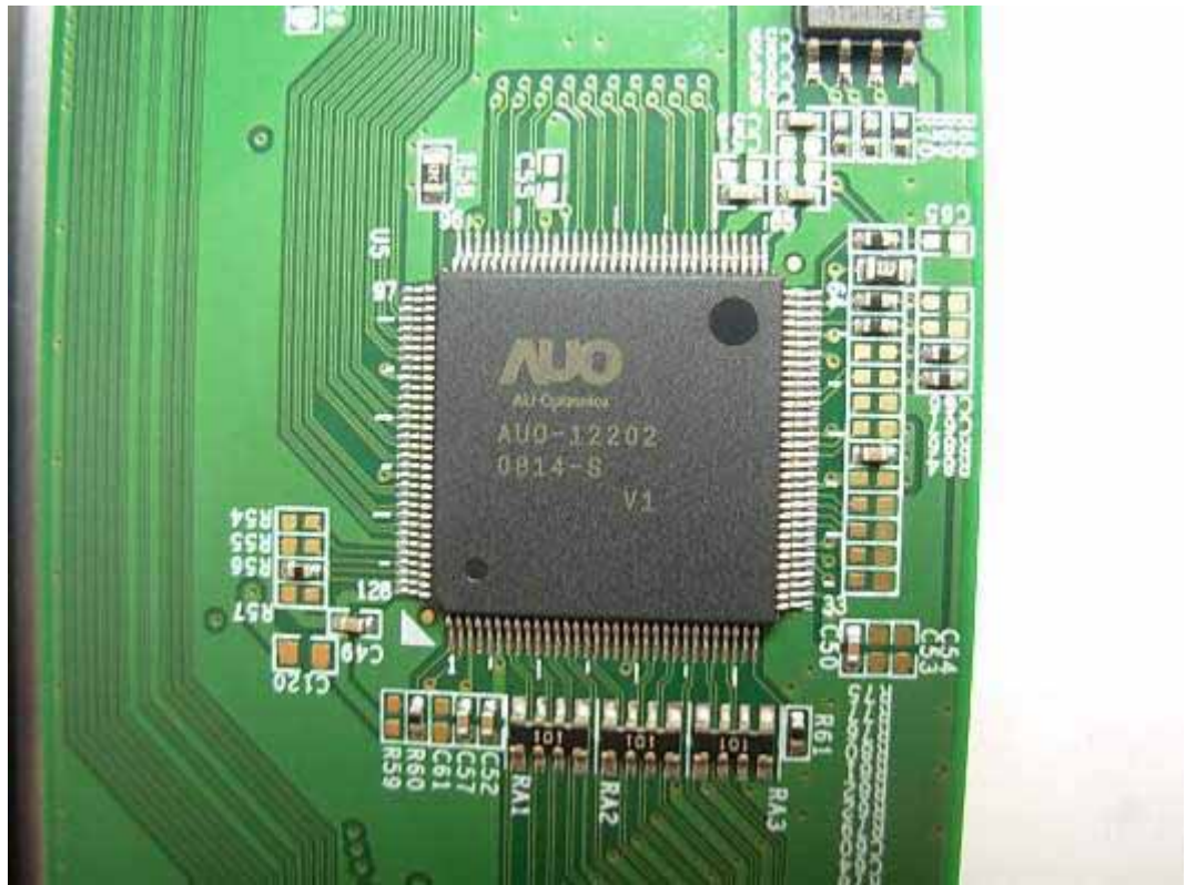
FIGURE 17 LCD MONITOR (M/N: W2442PAT) CHIP ON LCD PANEL MAIN BOARD
