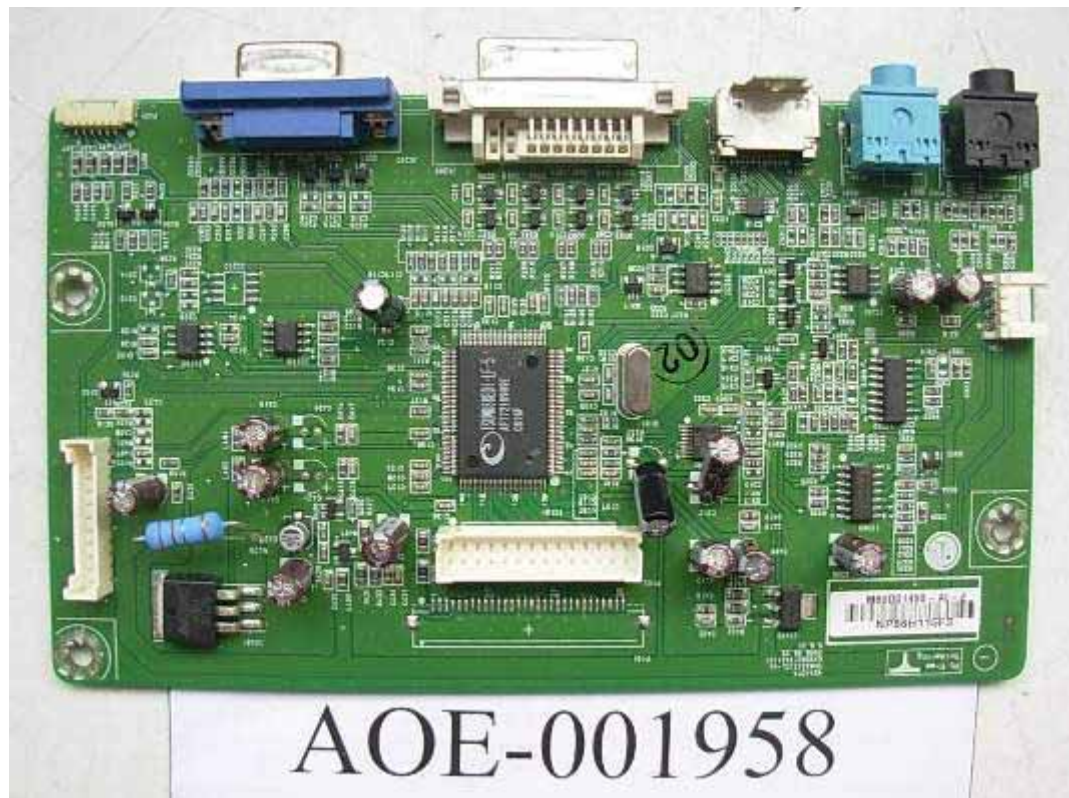
FIGURE 7 LCD MONITOR (M/N: W2442PAT) MAIN BOARD (COMPONENT SIDE)
