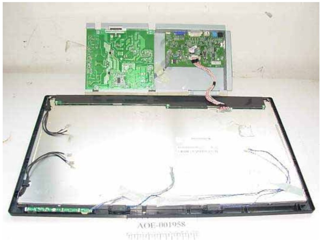
FIGURE 4 LCD MONITOR (M/N: W2442PAT) BOARDS REMOVED
