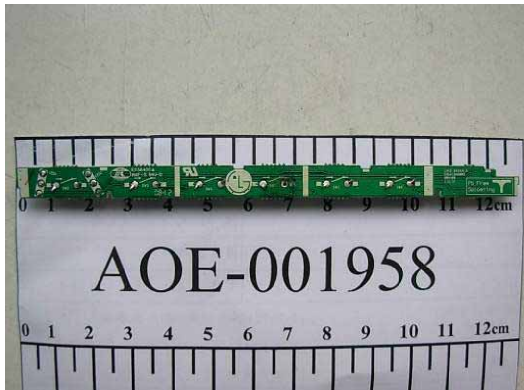
FIGURE 3 LCD MONITOR (M/N: W2442PAT) KEY BOARD (SOLDERED SIDE)
