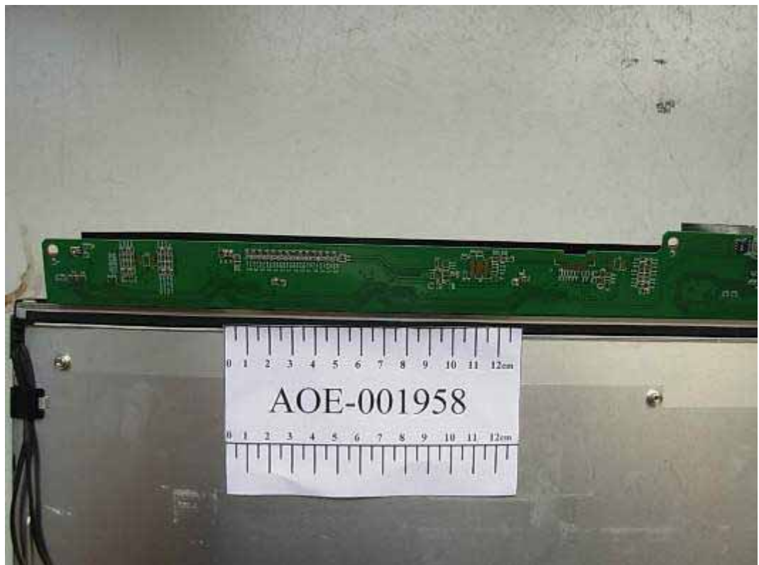
FIGURE 14 LCD MONITOR (M/N: W2442PAT) LCD PANEL MAIN BOARD (COMPONENT SIDE) 2
