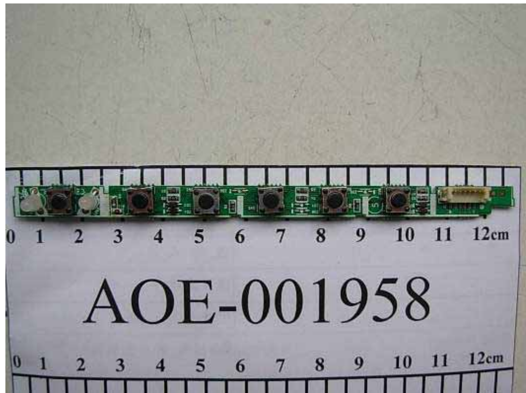
FIGURE 2 LCD MONITOR (M/N: W2442PAT) KEY BOARD (COMPONENT SIDE)
