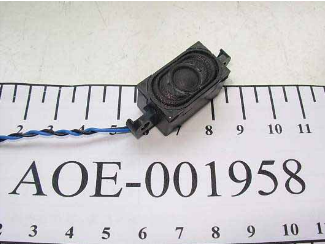
FIGURE 11 LCD MONITOR (M/N: W2442PAT) SPEAKER
