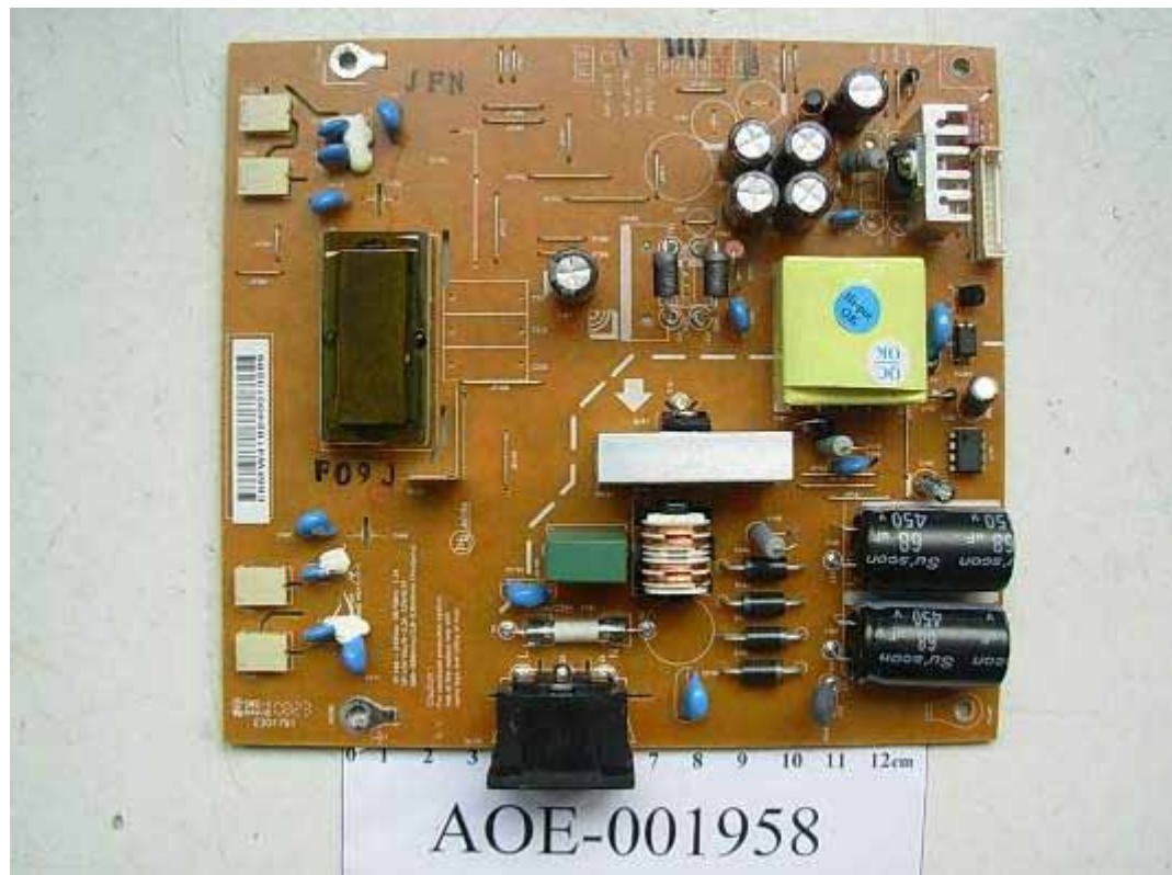
FIGURE 5 LCD MONITOR (M/N: W2442PAT) POWER BOARD (COMPONENT SIDE)
