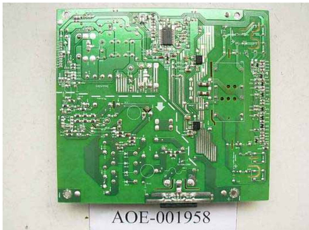
FIGURE 6 LCD MONITOR (M/N: W2442PAT) POWER BOARD (SOLDERED SIDE)
