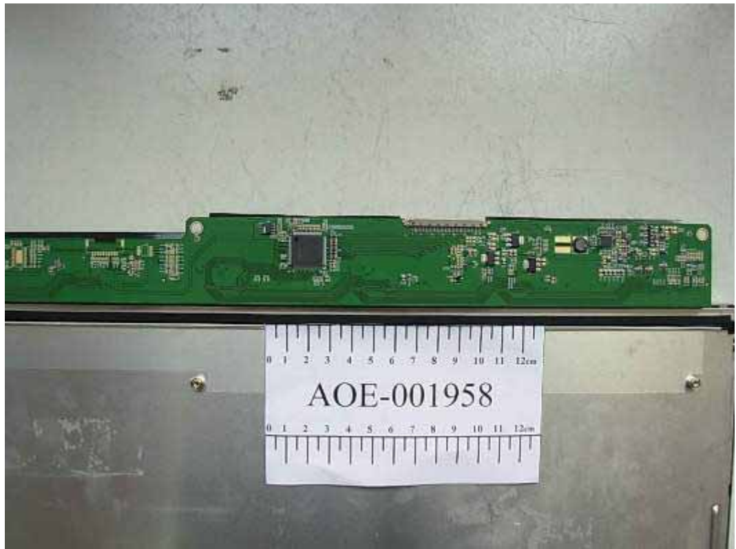
FIGURE 13 LCD MONITOR (M/N: W2442PAT) LCD PANEL MAIN BOARD (COMPONENT SIDE) 1
