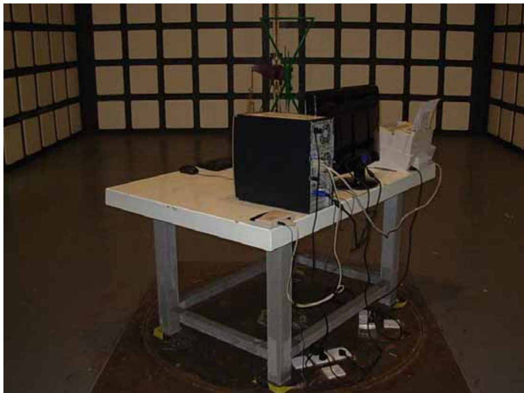
SETUP WITH MAXIMUM DETECTED EMISSION AT VERTICAL POLARIZATION (VGA 1920*1200@60Hz)
