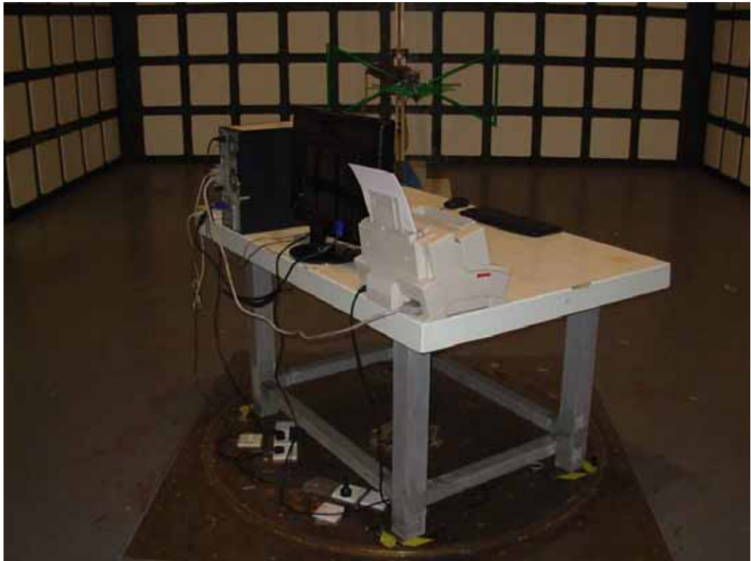
SETUP WITH MAXIMUM DETECTED EMISSION AT HORIZONTAL POLARIZATION (VGA 1920*1200@60Hz)
