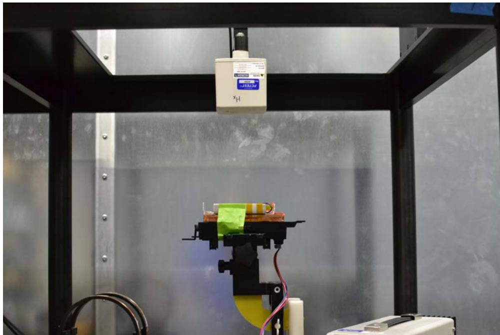
E/H Field Measurement on EUT Side "E" (20cm)
