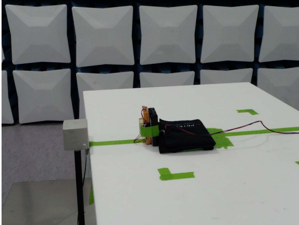
Figure 10. E-/H-Field Measurement (Position E)
