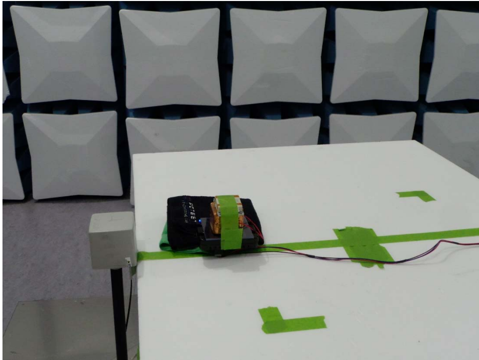
Figure 11. E-/H-Field Measurement (Position A)
