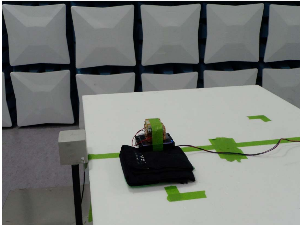
Figure 13. E-/H-Field Measurement (Position C)
