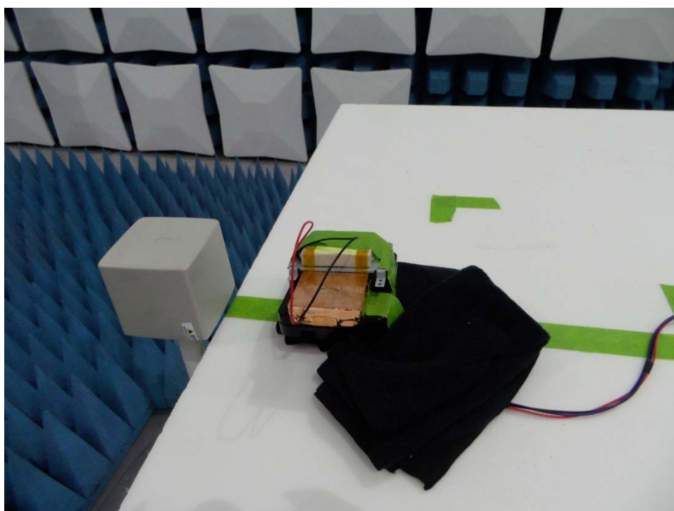
Figure 9. E-/H-Field Measurement (Position D)
