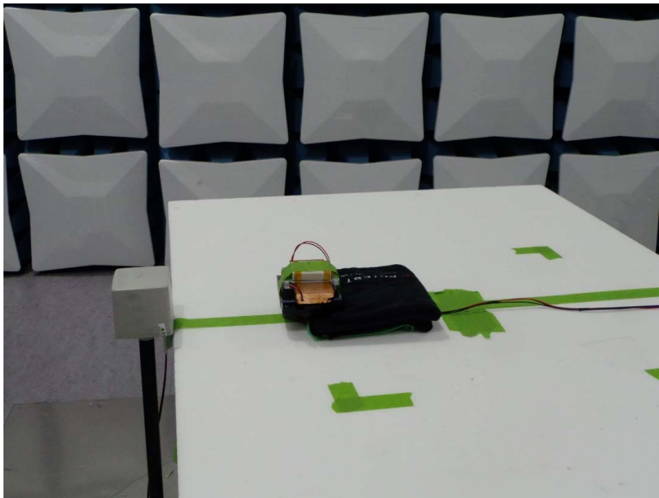
Figure 7. E-/H-Field Measurement (Position B)
