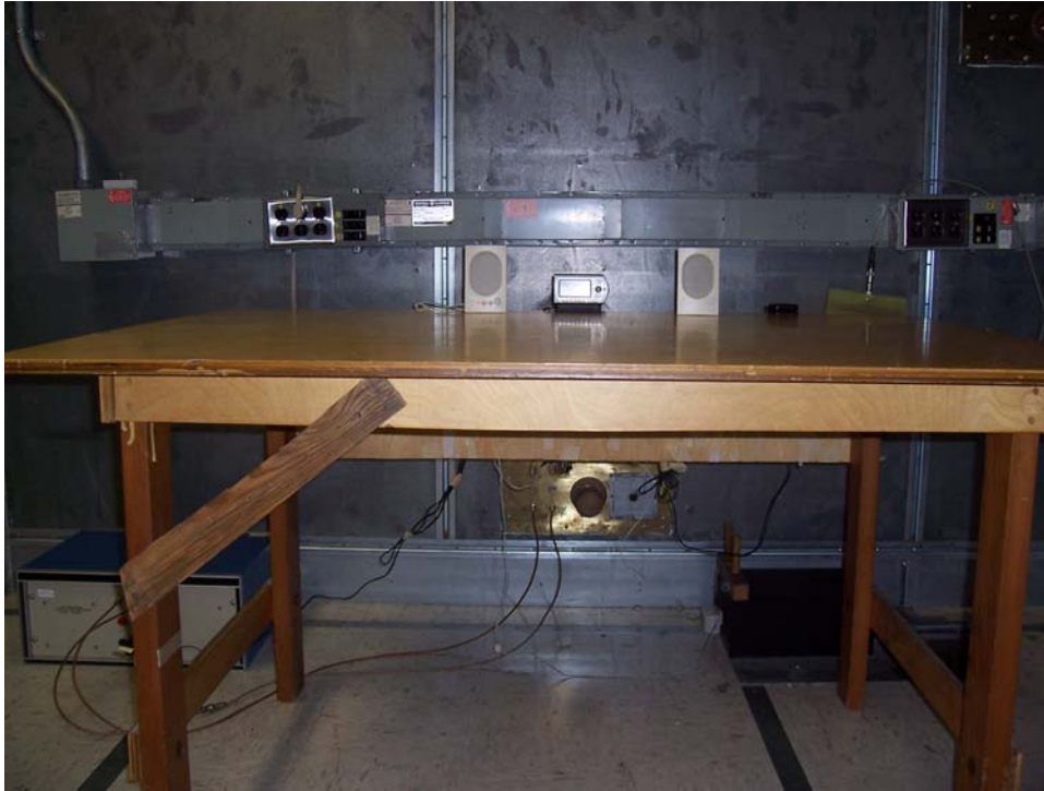
Conducted Emissions Test Setup, View 1
