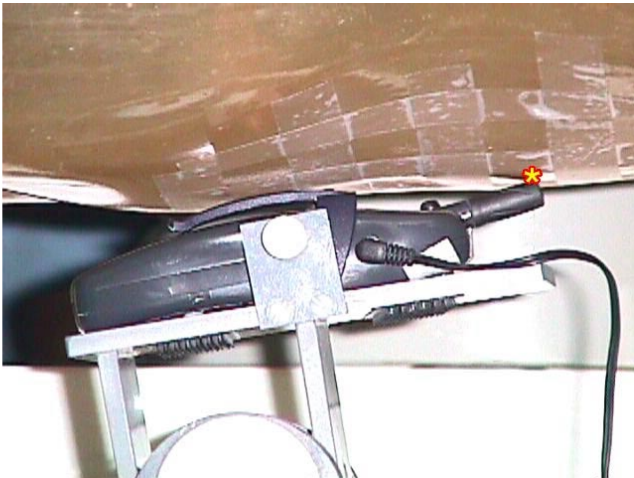
< Close-up view – Tip of the antenna in contact with the phantom >
