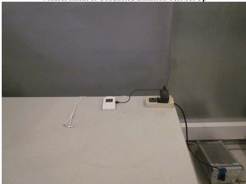
Measurement of Conducted Emission Test Set Up
