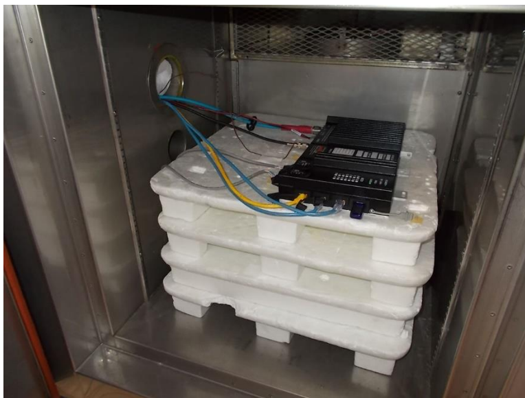
Conducted RF In Temperature Chamber
